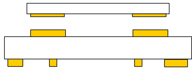
Figure 20. Correct PCB Top Metal Pattern Under Package
