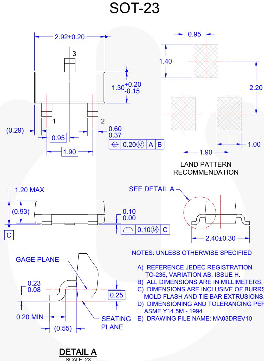
Figure1. 3-LEAD, SOT23, JEDEC TO-236, LOW PROFILE (ACTIVE)
