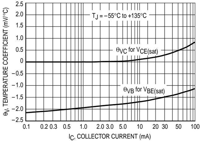
Figure 5. Temperature Coefficients
