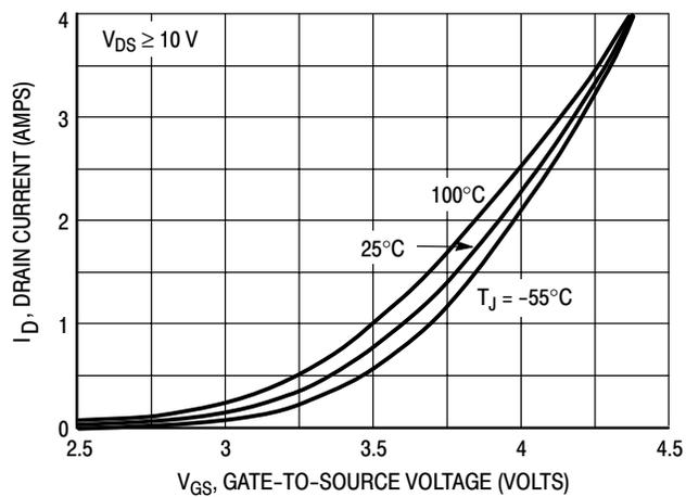
Figure 2. Transfer Characteristics
