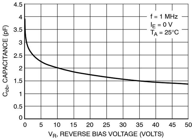
Figure 29. Output Capacitance
