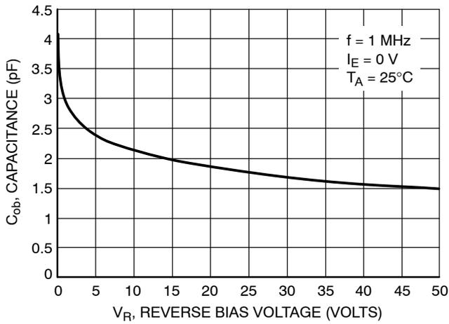
Figure 24. Output Capacitance
