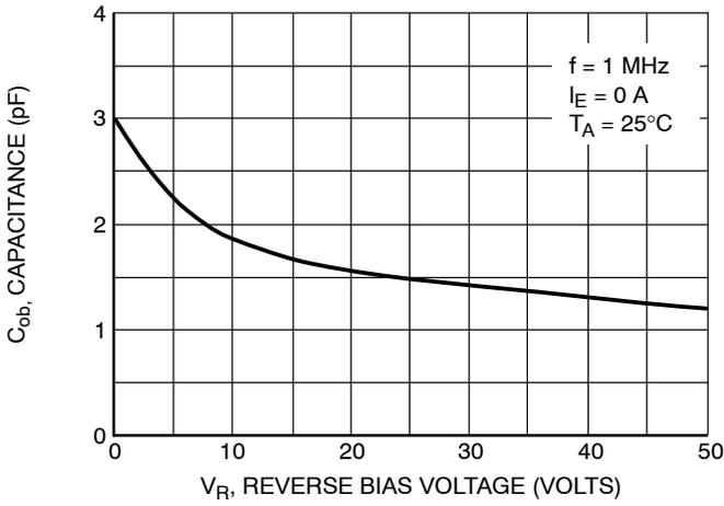
Figure 9. Output Capacitance
