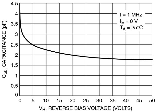
**Figure 39. Output Capacitance**
