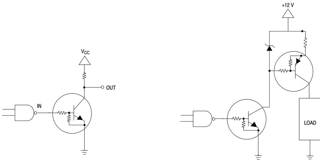
Figure 63. Open Collector Inverter: Inverts the Input Signal
