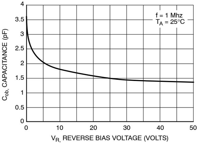
Figure 59. Output Capacitance
