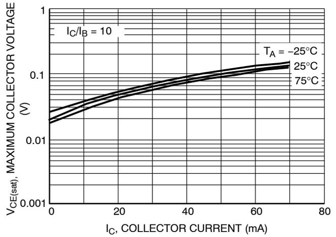
Figure 2. V<sub>CE(sat)</sub> vs. I<sub>C</sub>
