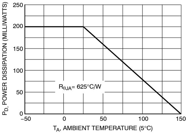
Figure 1. Derating Curve
