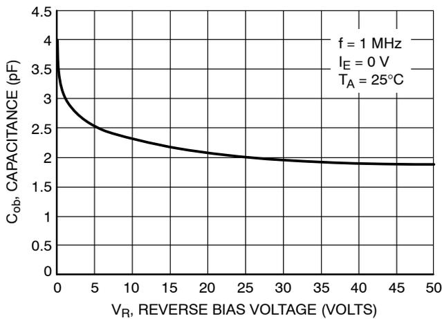
Figure 34. Output Capacitance
