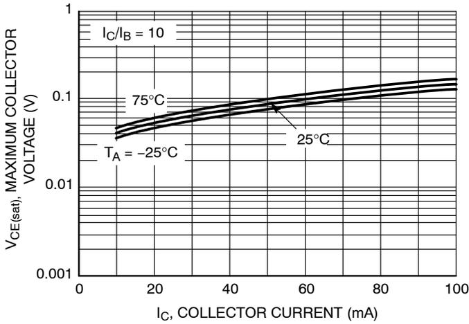
Figure 57.  $V_{CE(sat)}$  vs.  $I_C$
