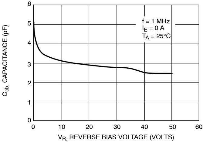
Figure 44. Output Capacitance
