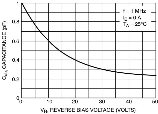
Figure 14. Output Capacitance
