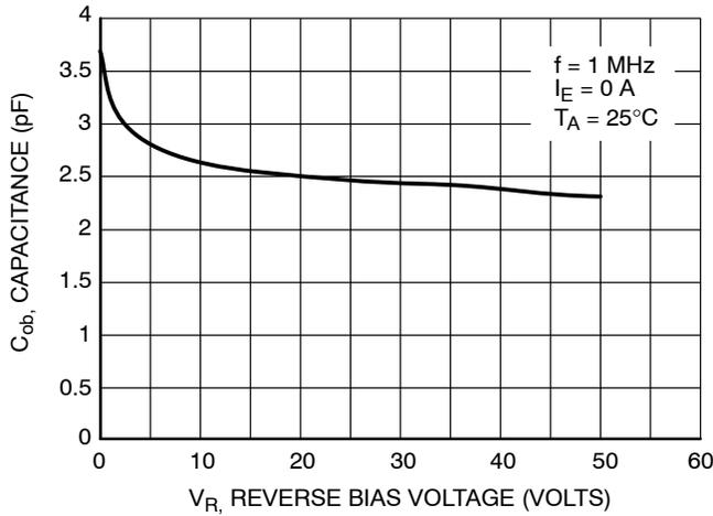
Figure 49. Output Capacitance
