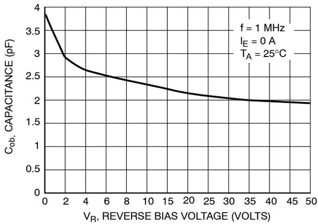
Figure 19. Output Capacitance
