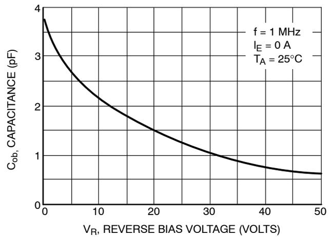
Figure 4. Output Capacitance
