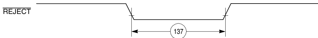
Figure 65. CAM Interface \overline{\text{REJECT}} Timing Diagram
