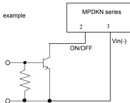
The voltage of maximum 20V appears in the ON/OFF pin at the time of pin opening.
