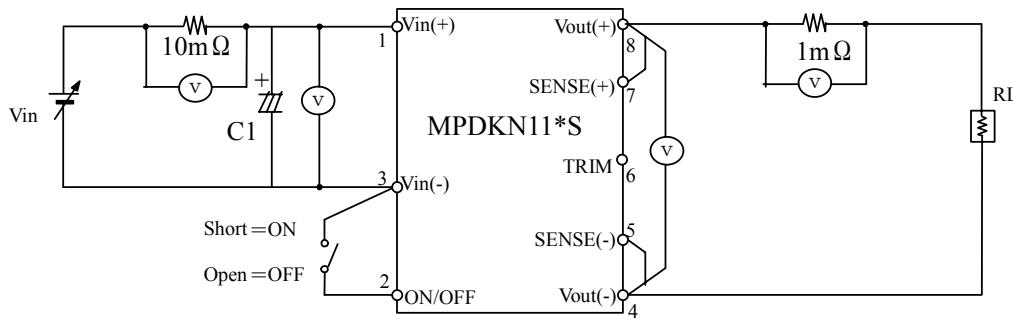
C1: Low Impedance Electrolytic Capacitor 33µF
