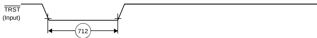
Figure 29. TRST Timing Diagram
