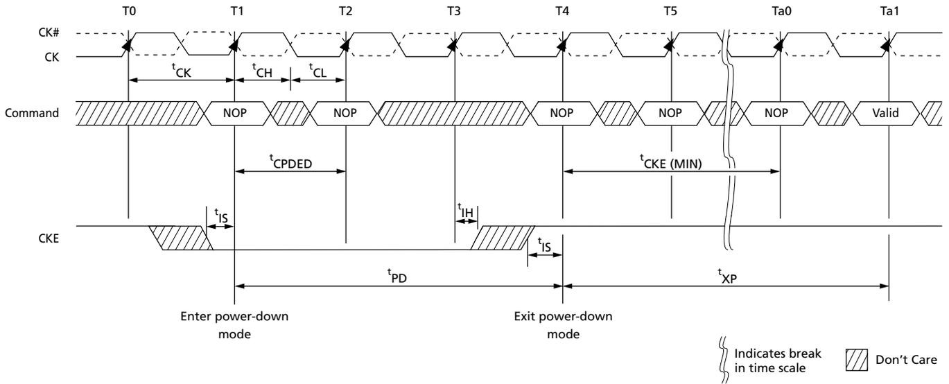
Figure 94: Precharge Power-Down (Slow-Exit Mode) Entry and Exit
