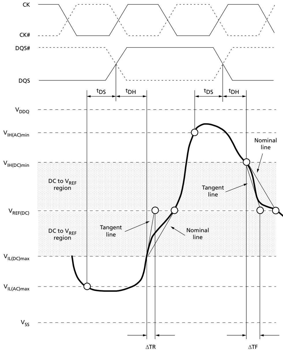
$$\text{Hold slew rate rising signal} = \frac{\text{Tangent line } (V_{REF(DC)} - V_{IL(DC)max})}{\Delta TR}$$
