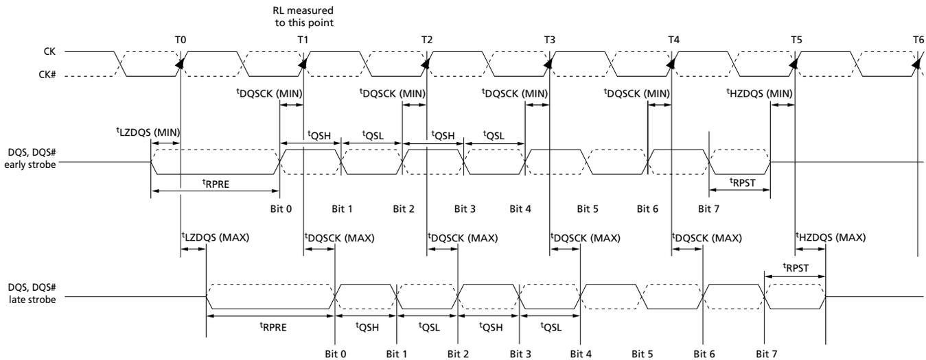
**Figure 75: Method for Calculating  $t_{HZ}$  and  $t_{LZ}$**
