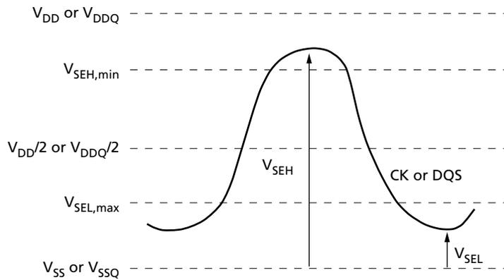
**Figure 15: Definition of Differential AC-Swing and  $t_{DVAC}$**
