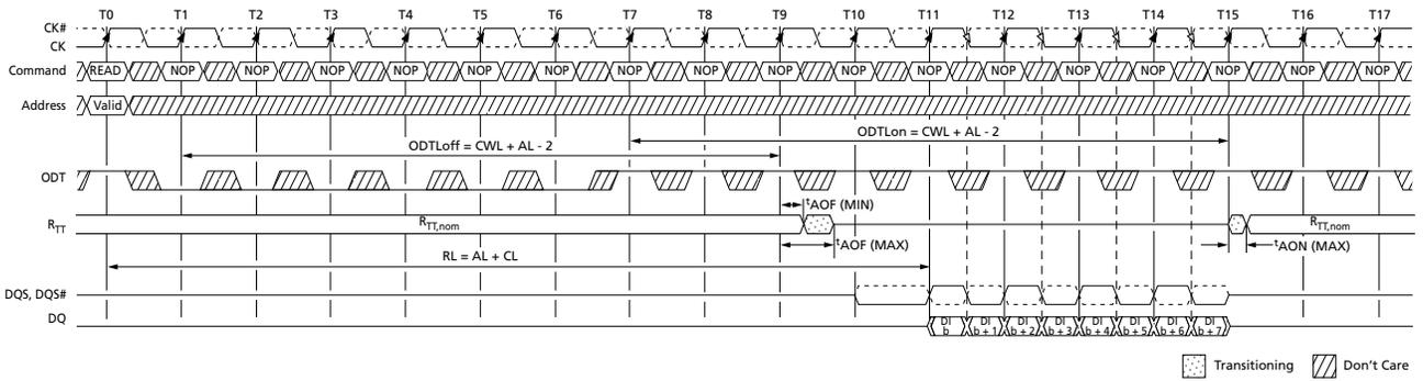
Note: 1. ODT must be disabled externally during READs by driving ODT LOW. For example,  $CL = 6$ ;  $AL = CL - 1 = 5$ ;  $RL = AL + CL = 11$ ;  $CWL = 5$ ;  $ODTL_{on} = CWL + AL - 2 = 8$ ;  $ODTL_{off} = CWL + AL - 2 = 8$ .  $R_{TT, nom}$  is enabled.  $R_{TT(WR)}$  is a "Don't Care."
