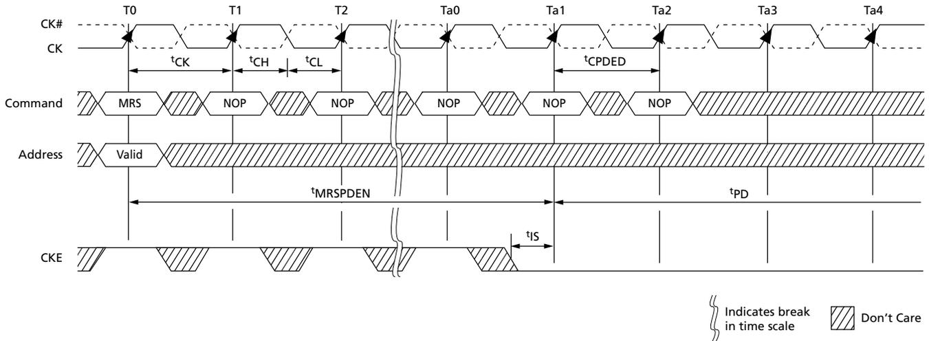
Figure 102: Power-Down Exit to Refresh to Power-Down Entry
