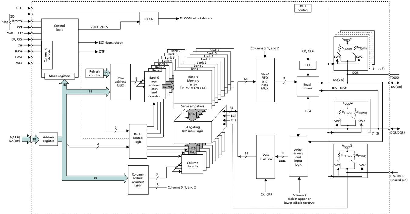
**Figure 4: 128 Meg x 16 Functional Block Diagram**
