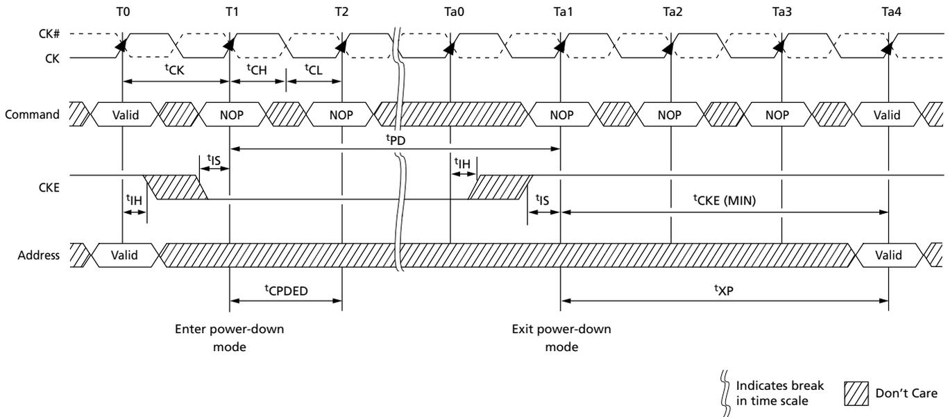
Figure 93: Precharge Power-Down (Fast-Exit Mode) Entry and Exit
