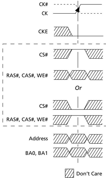
**Figure 51: Power-Down Mode (Active or Precharge)**
