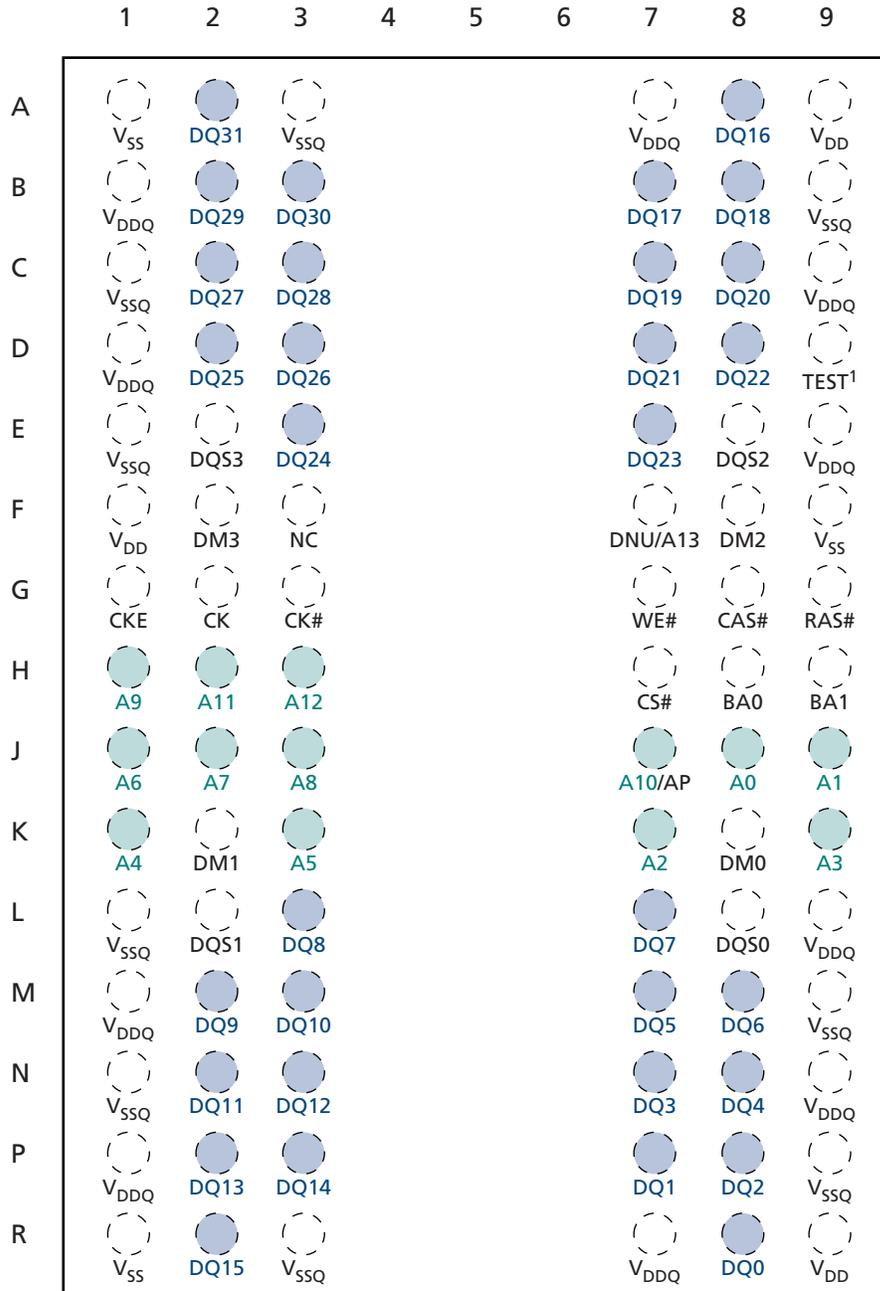
Note: 1. D9 is a test pin that must be tied to V<sub>SS</sub> or V<sub>SSQ</sub> in normal operations.
