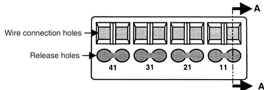
**Fig. 2 Wire Connection Holes and Release Holes**
