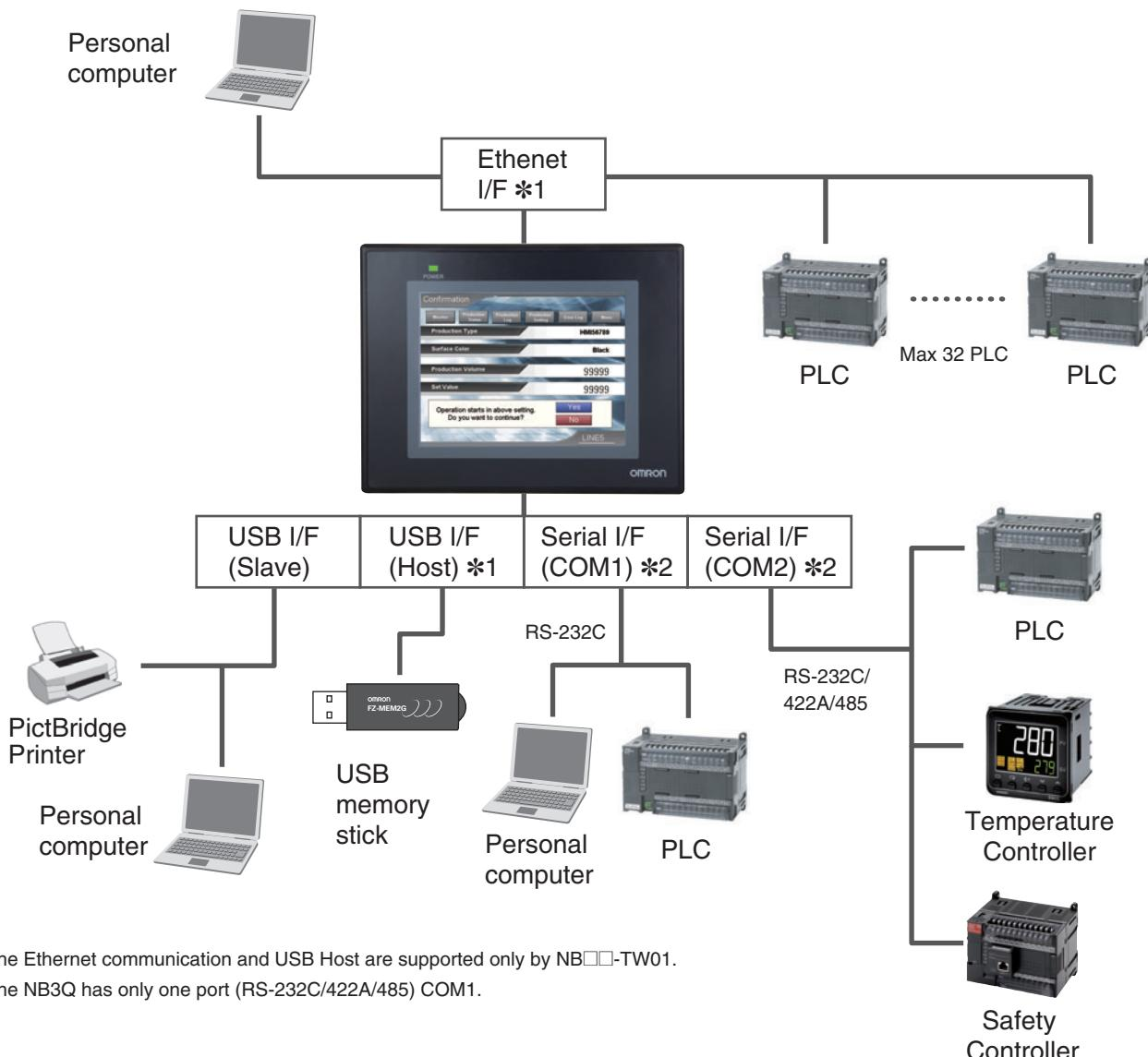
\*1. The Ethernet communication and USB Host are supported only by NB□□-TW01.
