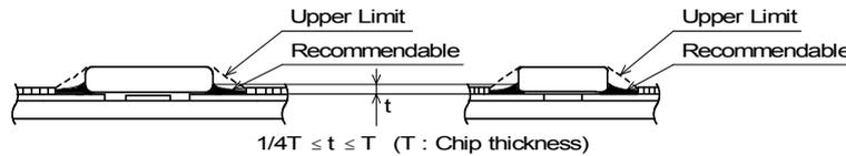
Accordingly increasing the solder volume, the mechanical stress to product is also increased. Excessive solder volume may cause the failure of mechanical or electrical performance.
