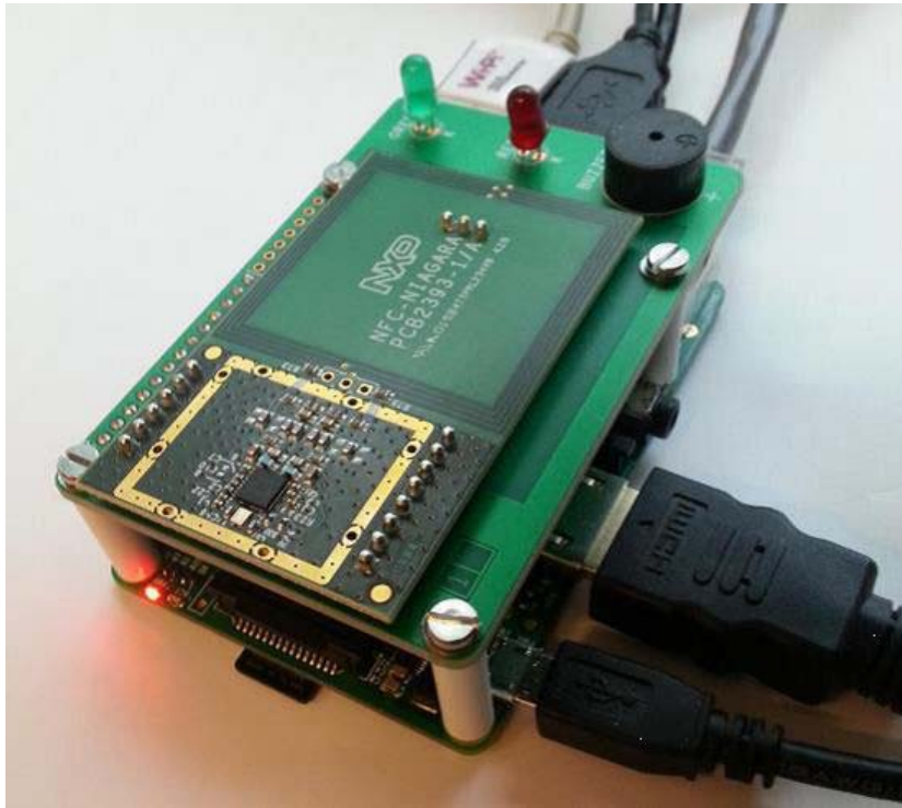
Figure 30: NFC Controller Assembly on Raspberry Pi Board
