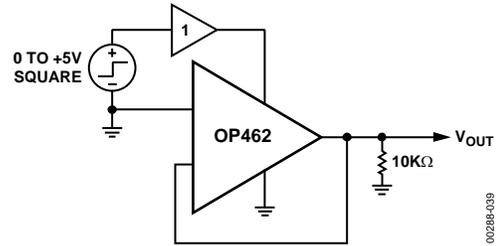
Figure 39. Test Circuit for Power-On Settling Time
