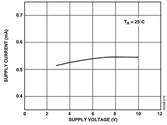
Figure 18. OP462 Supply Current/Amplifier vs. Supply Voltage
