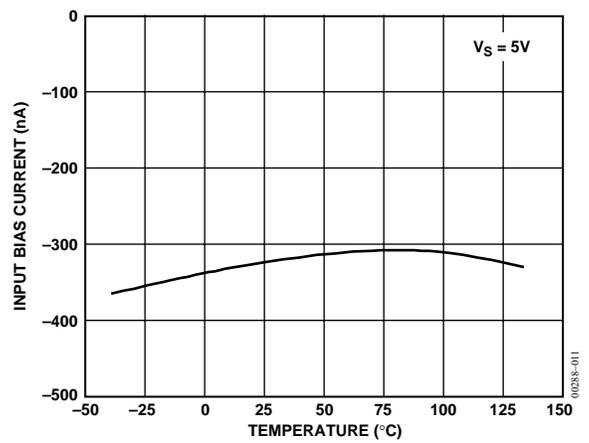
Figure 11. OP462 Input Bias Current vs. Temperature
