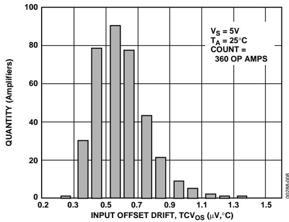
Figure 8. OP462 Input Offset Voltage Drift ( $TCV_{os}$ )
