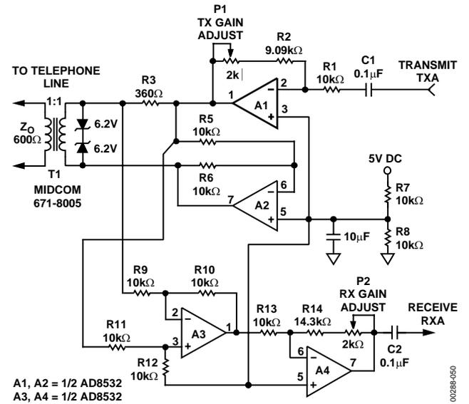
Figure 50. Single-Supply Direct Access Arrangement for Modems
