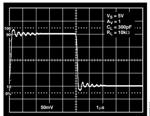
Figure 41. A Photo of a Ringing Square Wave
