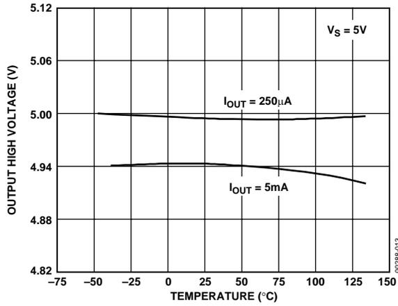
Figure 13. OP462 Output High Voltage vs. Temperature
