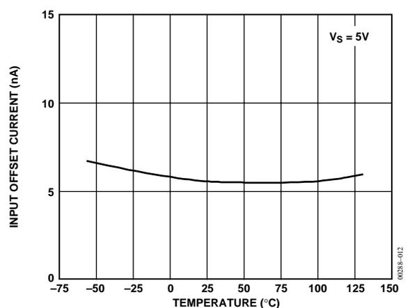
Figure 12. OP462 Input Offset Current vs. Temperature
