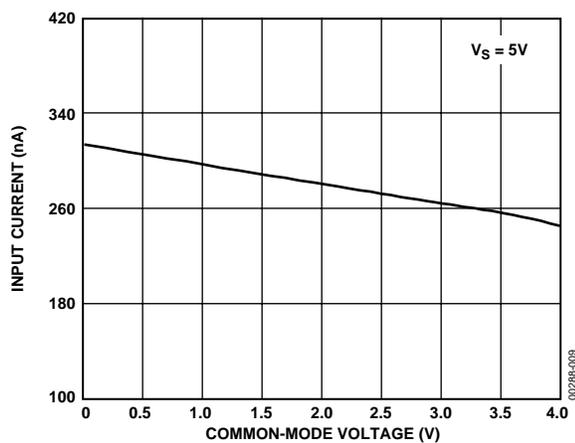
Figure 9. OP462 Input Bias Current vs. Common-Mode Voltage
