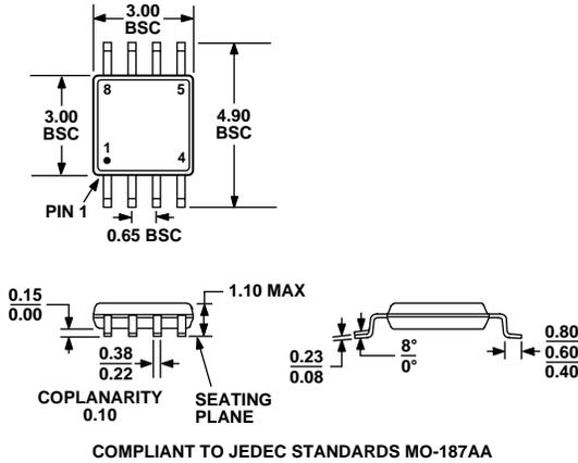
Figure 52. 8-Lead Mini Small Outline Package [MSOP] (RM-8)
