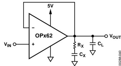
Figure 40. Snubber Network Compensation for Capacitive Loads
