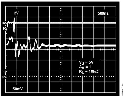
Figure 38. Oscilloscope Photo of  $V_S$  and  $V_{OUT}$
