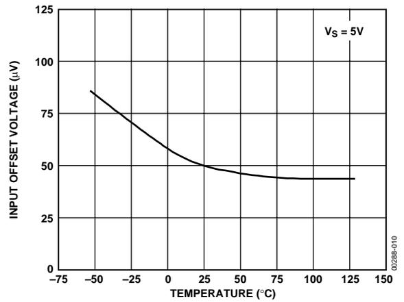
Figure 10. OP462 Input Offset Voltage vs. Temperature
