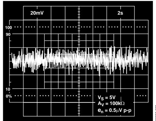
Figure 29. 0.1 Hz to 10 Hz Noise
