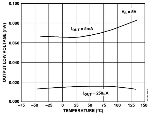
Figure 14. OP462 Output Low Voltage vs. Temperature
