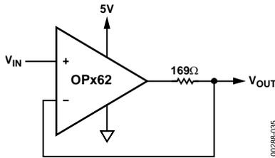
Figure 35. Output Short-Circuit Protection
