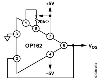
Figure 34. Offset Adjustment Schematic
