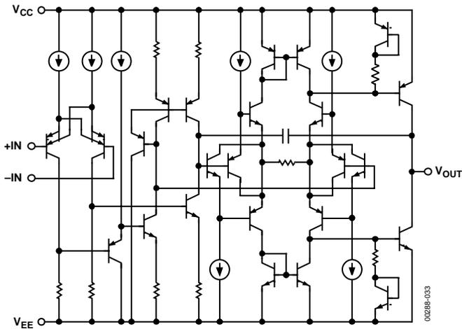
Figure 33. Simplified Schematic
