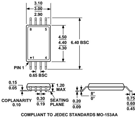
Figure 53. 8-Lead Thin Shrink Small Outline Package [TSSOP] (RU-8)
