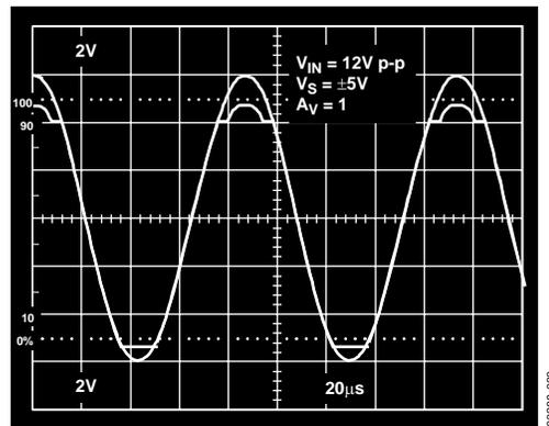
Figure 30. No Phase Reversal ( $V_{IN} = 12V$  p-p,  $V_S = \pm 5V$ ,  $A_V = 1$ )
