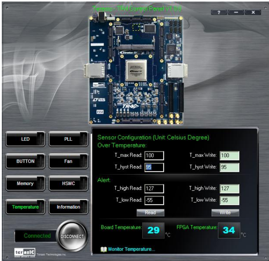
Figure 3-9 Accessing the Temperature Sensor through Control Panel
