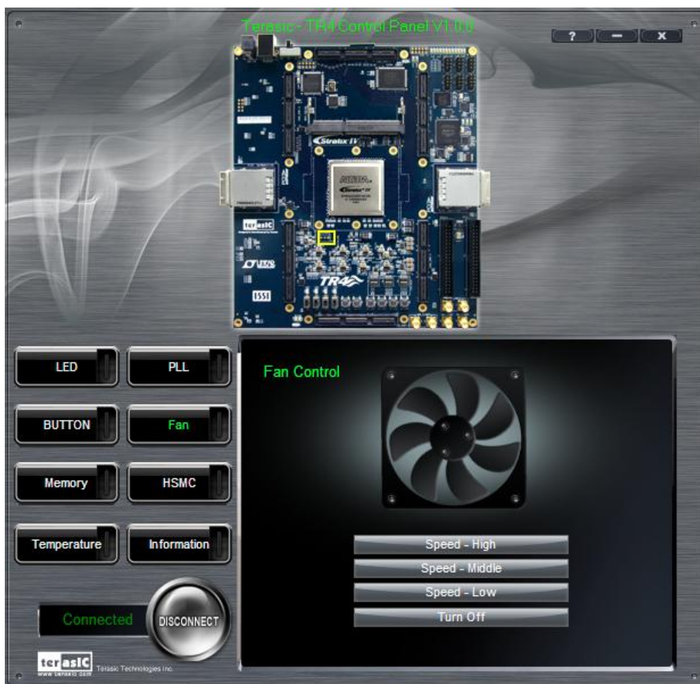
Figure 3-12 Fan Control of the TR4
