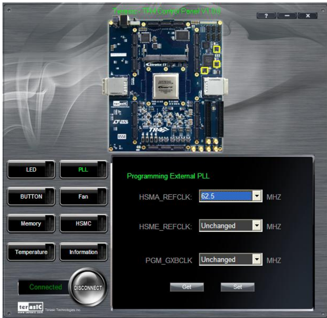
Figure 3-10 Programmable External PLL Configured through Control Panel
