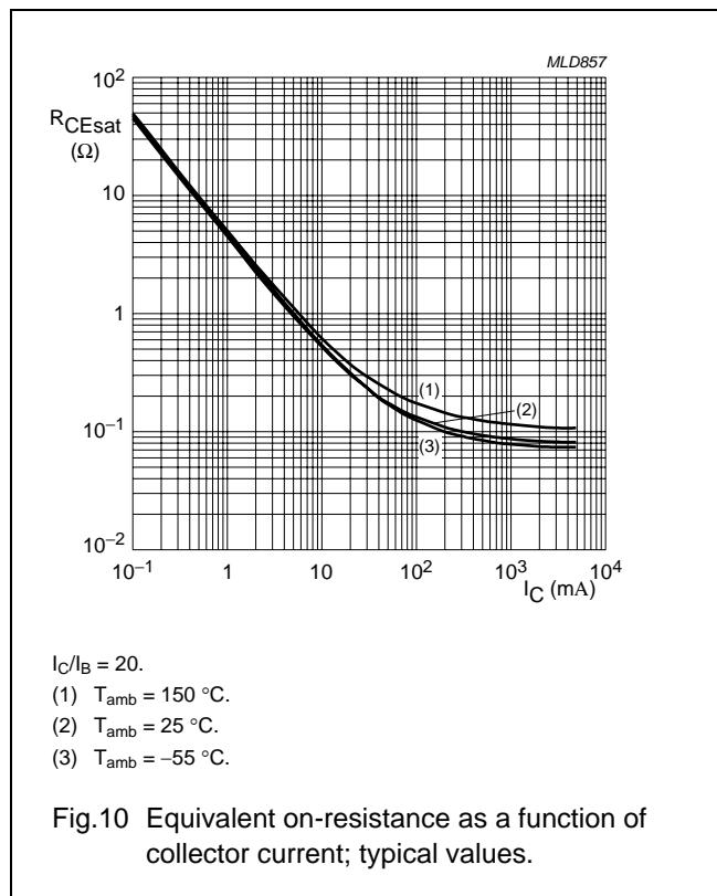
20 V NPN low  $V_{CEsat}$  transistor
