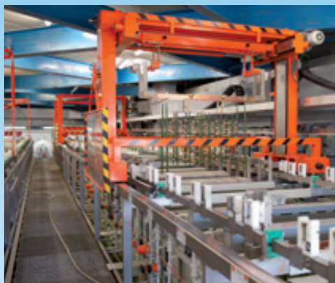
Surface treatment, chrome plating
