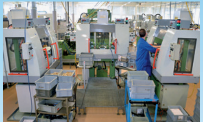
Automatic reworking of female contacts
