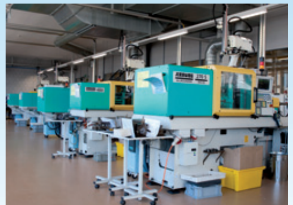
Injection of insulators
