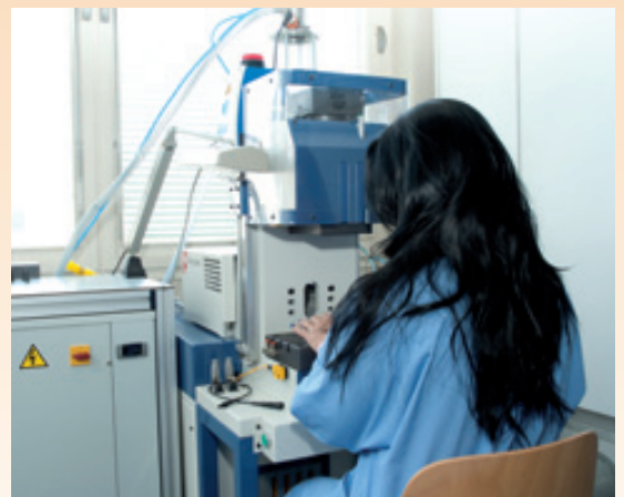
Over-moulding on cable
