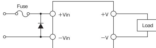
Figure 1-5: Protection for Reversed Connection of Input
