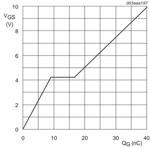
$I_D = 40$  A;  $V_{DD} = 15$  V
