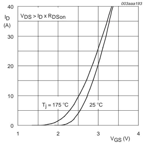
$T_j = 25\text{ }^\circ\text{C}$  and  $175\text{ }^\circ\text{C}$ ;  $V_{DS} > I_D \times R_{DSon}$
