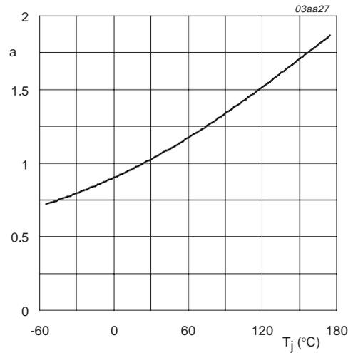
$$a = \frac{R_{DSon}}{R_{DSon(25^\circ\text{C})}}$$
