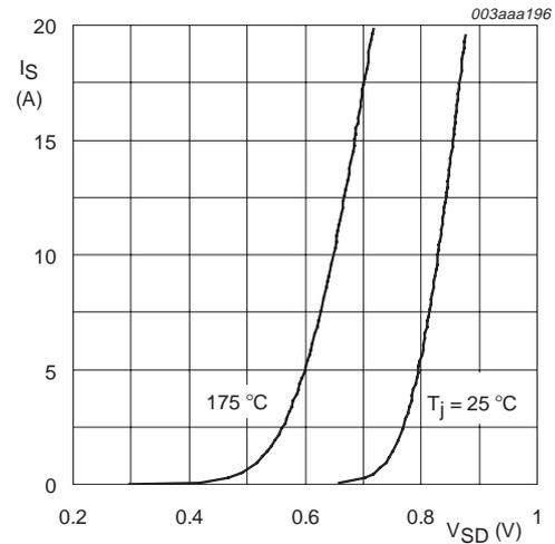
$T_j = 25 \text{ }^{\circ}C \text{ and } 175 \text{ }^{\circ}C; V_{GS} = 0 \text{ V}$
