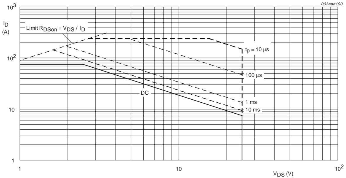
T<sub>mb</sub> = 25 °C; I<sub>DM</sub> is single pulse
