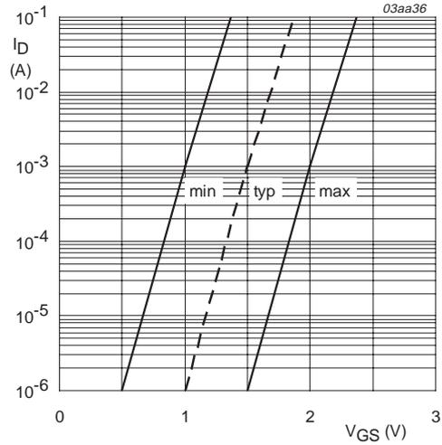
$T_j = 25 \text{ }^{\circ}C; V_{DS} = 5 \text{ V}$
