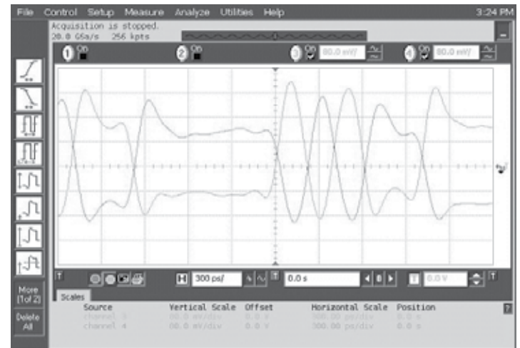
Data Waveforms, 3.0Gbps (left) & 6.0Gbps (right)
