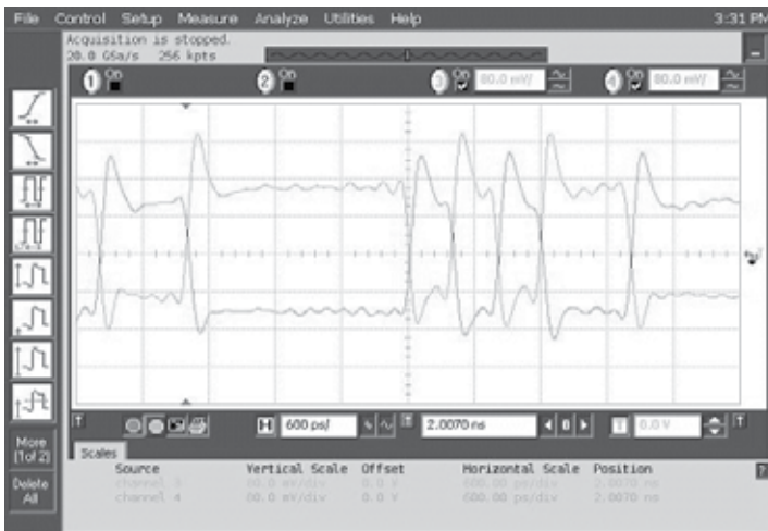
Data Waveforms, 3.0Gbps (left) & 6.0Gbps (right)
