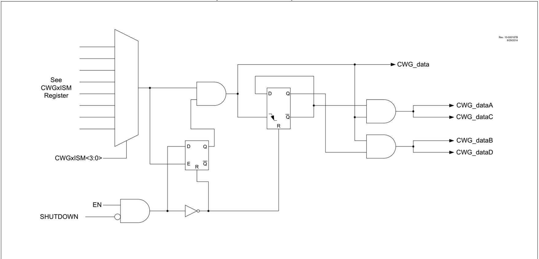
**FIGURE 28-3: SIMPLIFIED CWG BLOCK DIAGRAM (FORWARD AND REVERSE FULL-BRIDGE MODES)**
