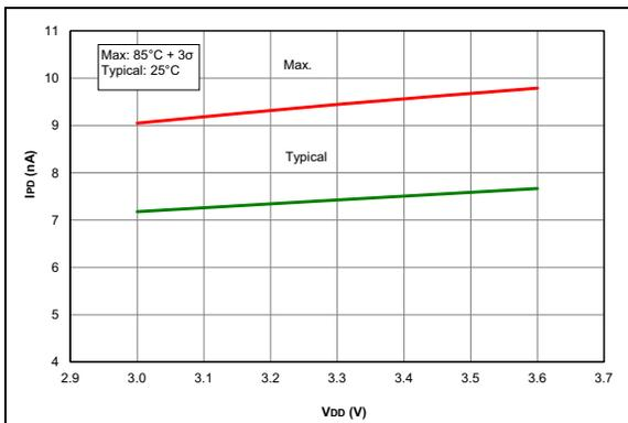
**FIGURE 36-33:**  $I_{PD}$ , Brown-Out Reset (BOR), BORV = 1, PIC16LF1615/9 Only.
