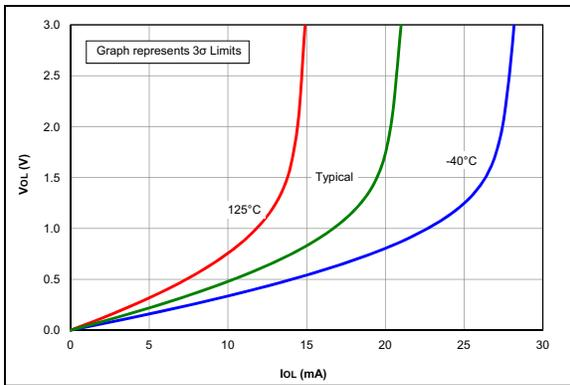
**FIGURE 36-48:**  $V_{OL}$  vs.  $I_{OL}$  Over Temperature,  $V_{DD} = 3.0V$ .
