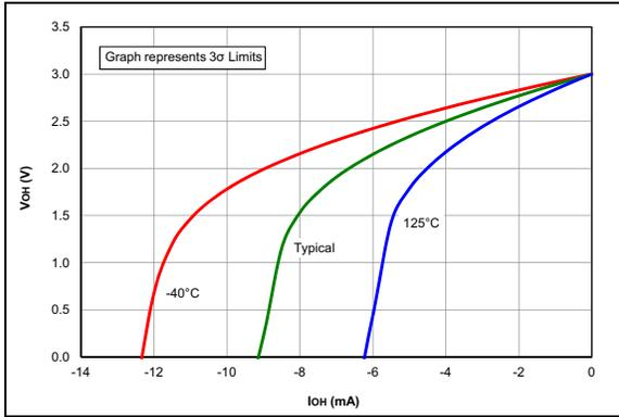
**FIGURE 36-47:**  $V_{OH}$  vs.  $I_{OH}$  Over Temperature,  $V_{DD} = 3.0V$ .
