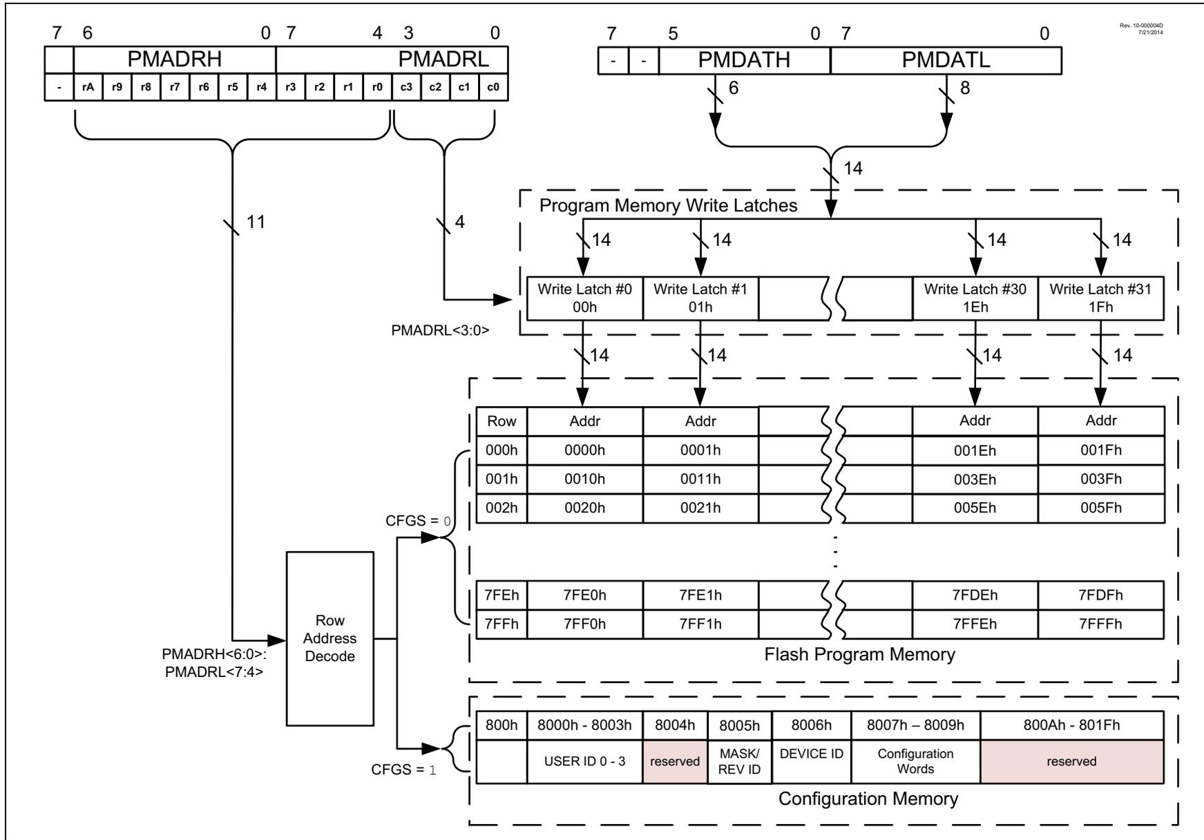
FIGURE 10-6: FLASH PROGRAM MEMORY WRITE FLOWCHART
