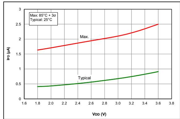
**FIGURE 36-29:**  $I_{PD}$ , Watchdog Timer (WDT), PIC16LF1615/9 Only.
