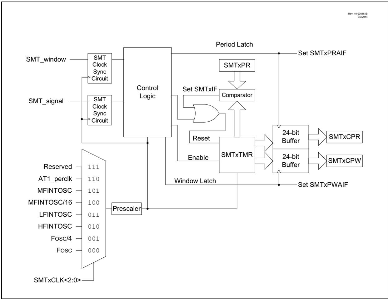
FIGURE 30-2: SMT SIGNAL AND WINDOW BLOCK DIAGRAM
