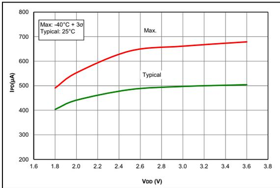
**FIGURE 36-41:**  $I_{PD}$ , Comparator, NP Mode ( $CxSP = 1$ ), PIC16LF1615/9 Only.
