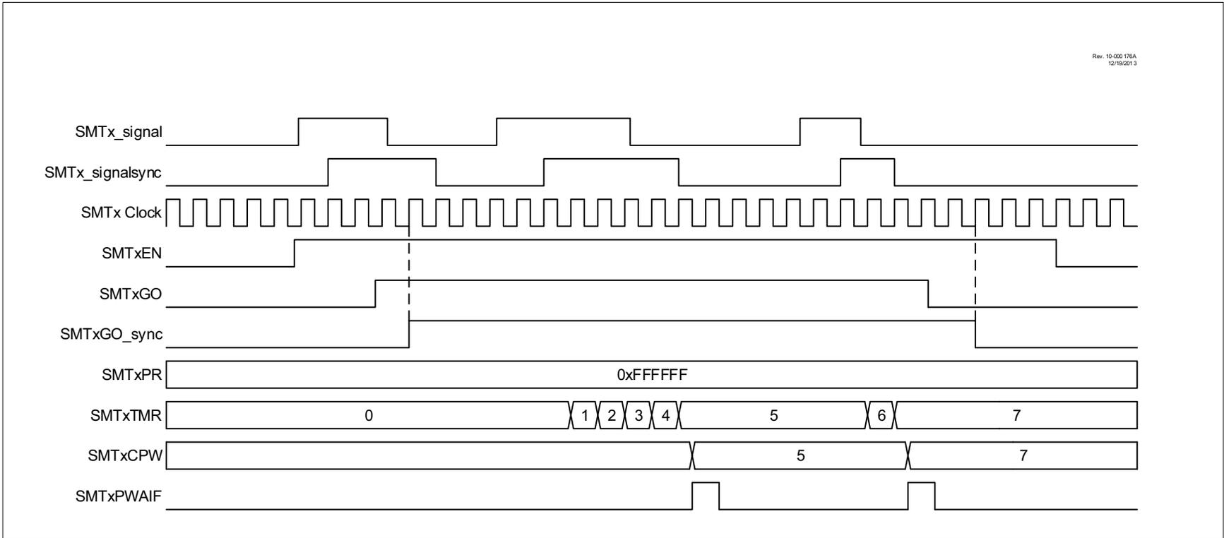
**FIGURE 30-5: GATED TIMER MODE SINGLE ACQUISITION TIMING DIAGRAM**
