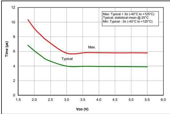
**FIGURE 36-68:** Wake From Sleep,  $V_{REGPM} = 0$ .
