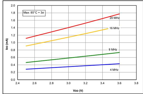
**FIGURE 36-22:**  $I_{DD}$  Maximum, HS Oscillator, PIC16LF1615/9 Only.
