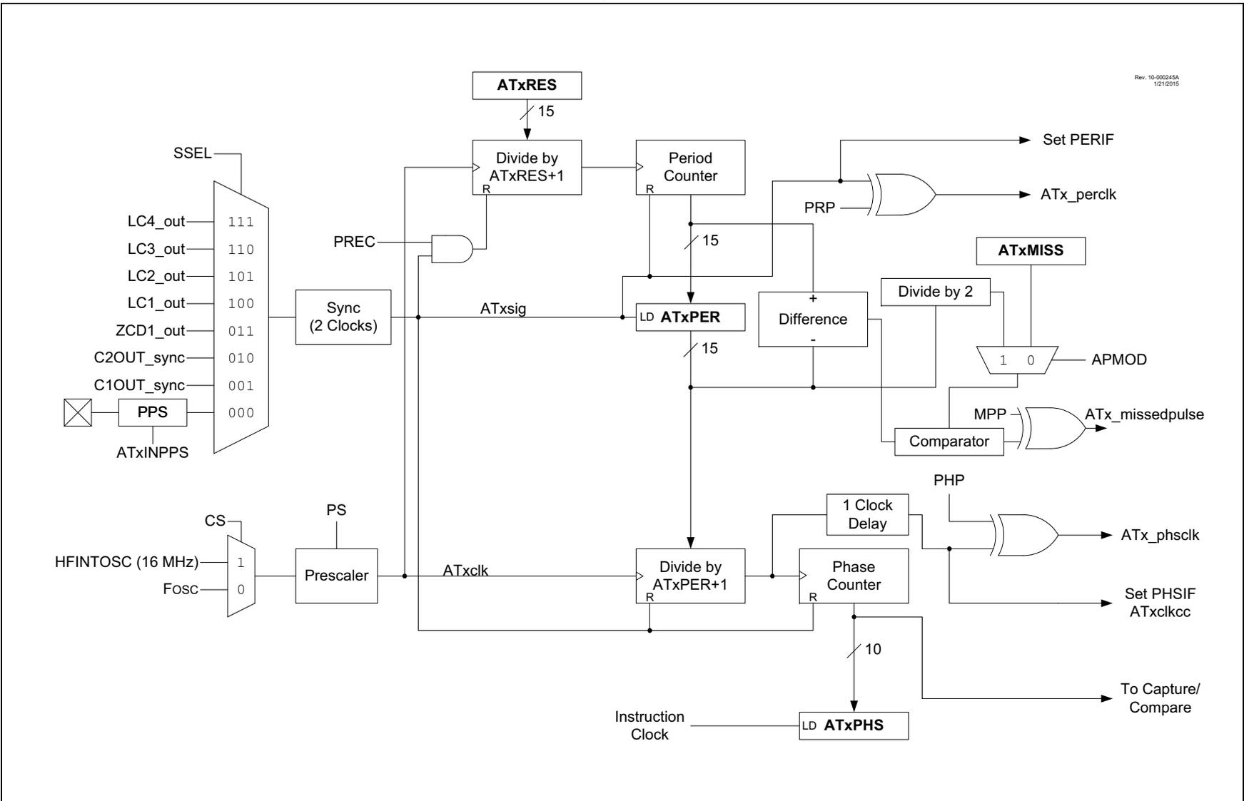
FIGURE 31-2: ANGULAR TIMER SIMPLIFIED BLOCK DIAGRAM, MULTI-PULSE MODE
