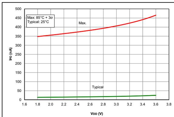
**FIGURE 36-39:**  $I_{PD}$ , ADC Non-Converting, PIC16LF1615/9 Only.
