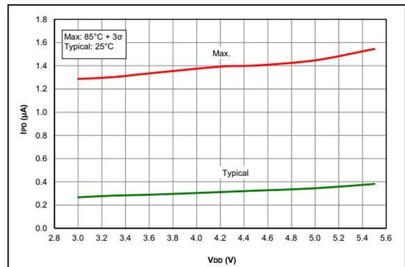
**FIGURE 36-36:**  $I_{PD}$ , LP Brown-Out Reset (LPBOR = 0), PIC16F1615/9 Only.
