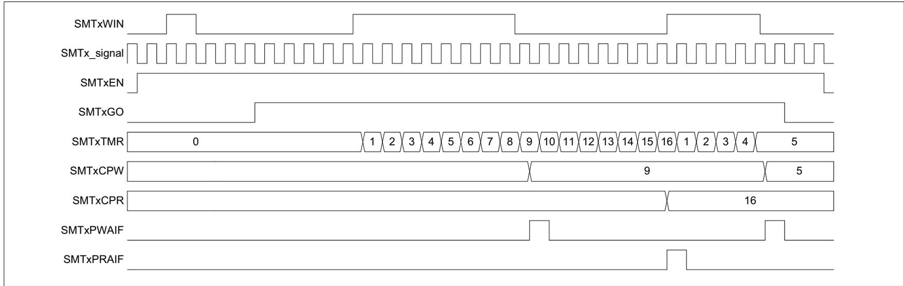
**FIGURE 30-22: WINDOWED COUNTER MODE SINGLE ACQUISITION TIMING DIAGRAM**
