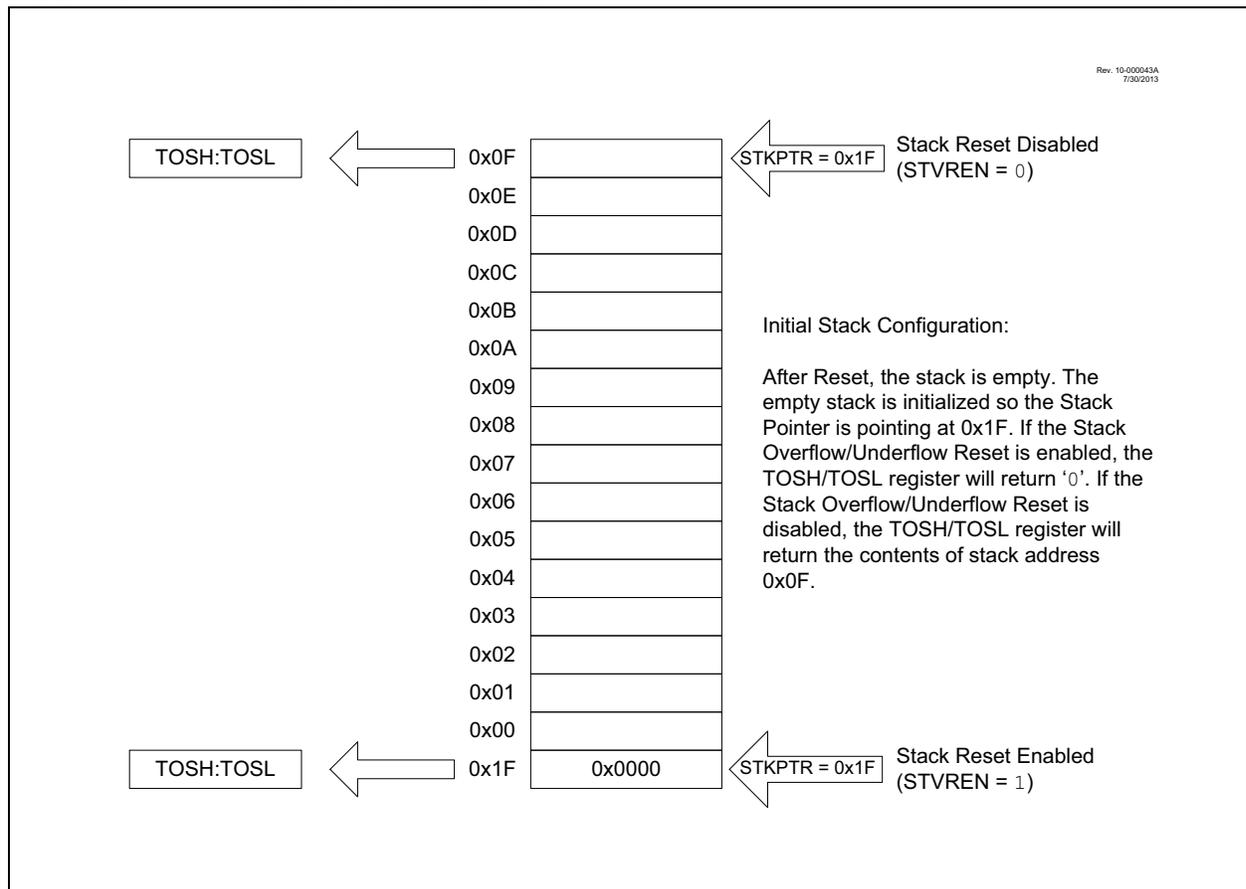
FIGURE 3-5: ACCESSING THE STACK EXAMPLE 2
