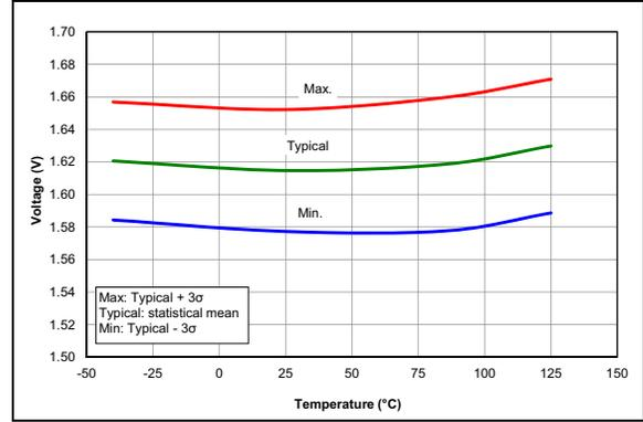
**FIGURE 36-65:** POR Release Voltage.
