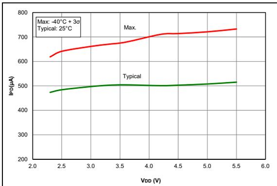
**FIGURE 36-42:**  $I_{PD}$ , Comparator, NP Mode ( $CxSP = 1$ ), PIC16F1615/9 Only.
