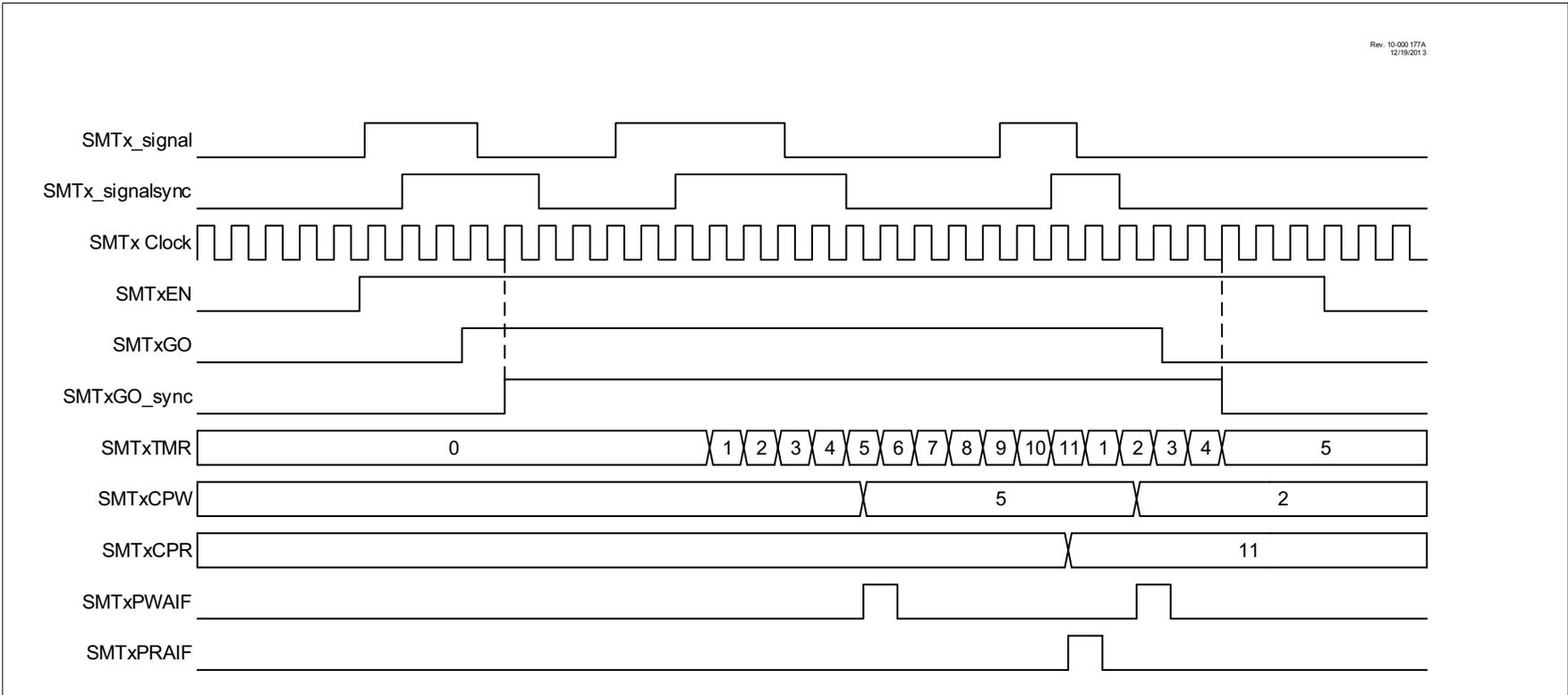
**FIGURE 30-7: PERIOD AND DUTY-CYCLE SINGLE ACQUISITION TIMING DIAGRAM**
