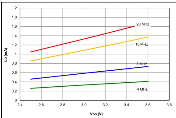
**FIGURE 36-21:**  $I_{DD}$  Typical, HS Oscillator, 25°C, PIC16LF1615/9 Only.
