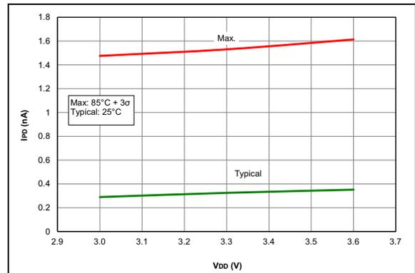
**FIGURE 36-35:**  $I_{PD}$ , LP Brown-Out Reset (LPBOR = 0), PIC16LF1615/9 Only.
