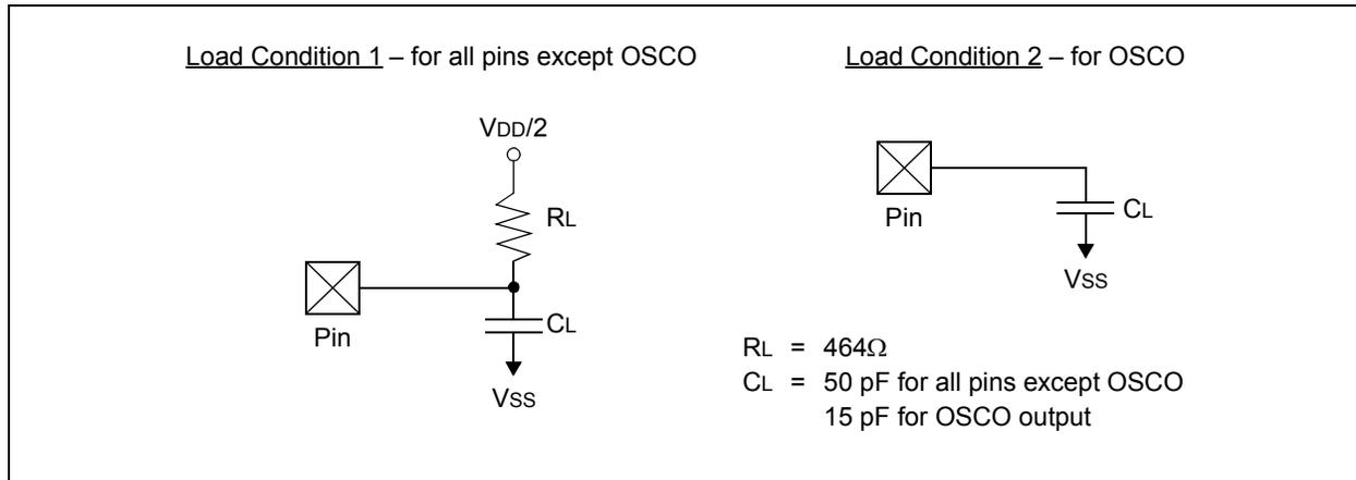
**TABLE 37-21: CAPACITIVE LOADING REQUIREMENTS ON OUTPUT PINS**
