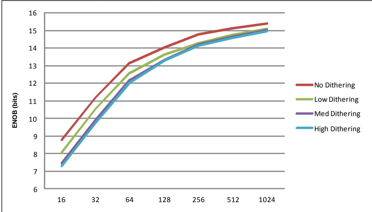
FIGURE 38-4: ENOB (SINAD) vs. OSR ( $V_{DD} = 3.3V$ ,  $V_{REF} = 2.0V$ ,  $F_{IN} = 25$  Hz,  $+25^{\circ}C$ )
