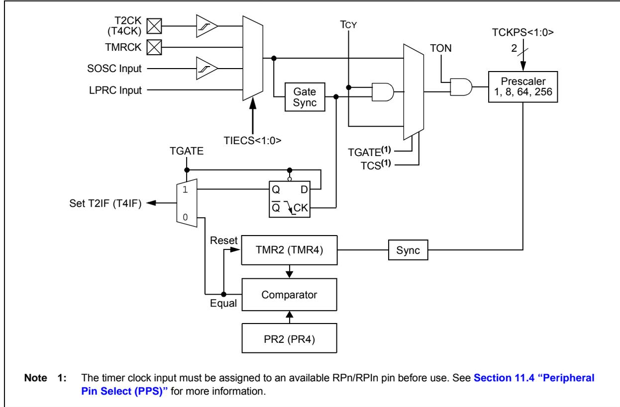
**FIGURE 13-3: TIMER3 AND TIMER5 (16-BIT ASYNCHRONOUS) BLOCK DIAGRAM**
