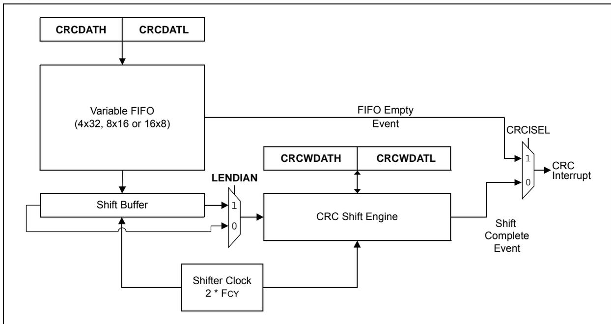
**FIGURE 24-2: CRC SHIFT ENGINE DETAIL**
