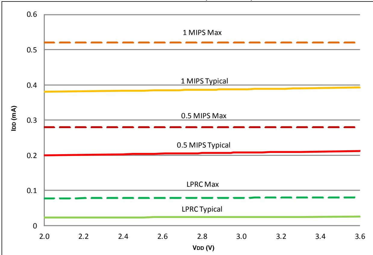
**FIGURE 38-9: 4 MIPS/16 MIPS I<sub>DD</sub> vs. V<sub>DD</sub> (RUN MODE)**
