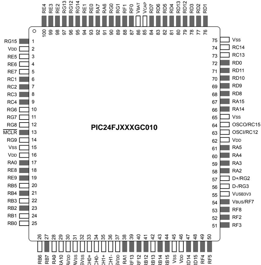
**Legend:** Shaded pins indicate pins tolerant to up to +5.5 VDC. See [Table 2](#) for a complete description of pin functions.
