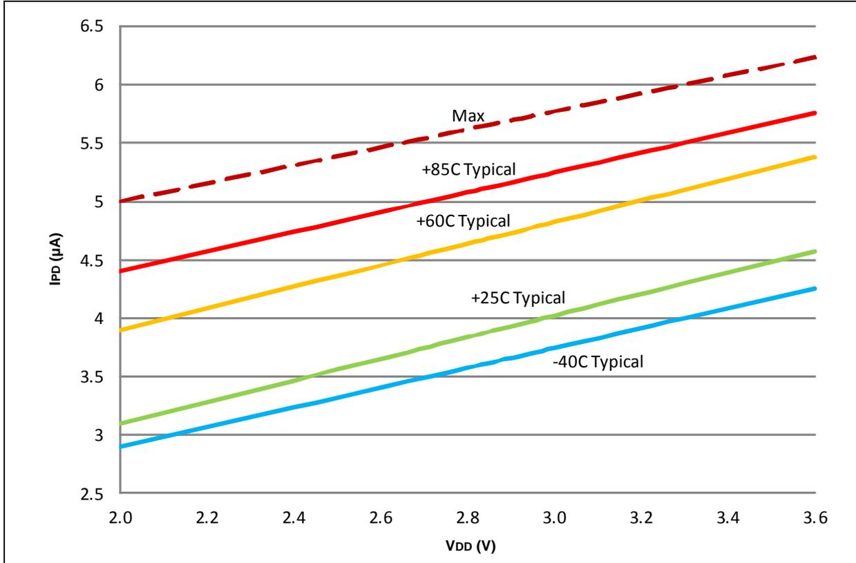
FIGURE 38-20: WDT WITH LPRC DELTA IPD vs. VDD
