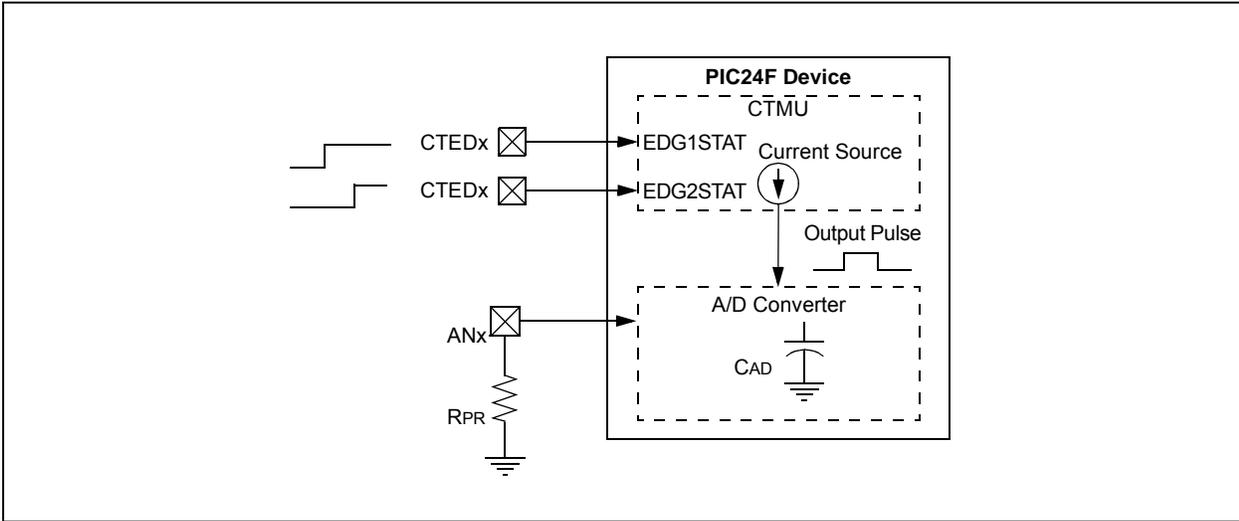
**FIGURE 32-4: TYPICAL CONNECTIONS AND INTERNAL CONFIGURATION FOR PULSE DELAY GENERATION**
