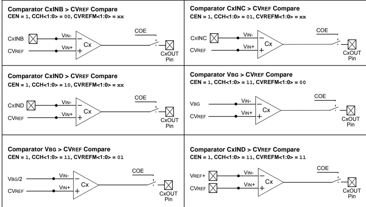
**FIGURE 30-4: INDIVIDUAL COMPARATOR CONFIGURATIONS WHEN CREF = 1 AND CVREFP = 1**
