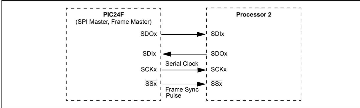
**FIGURE 16-6: SPIx MASTER, FRAME SLAVE CONNECTION DIAGRAM**
