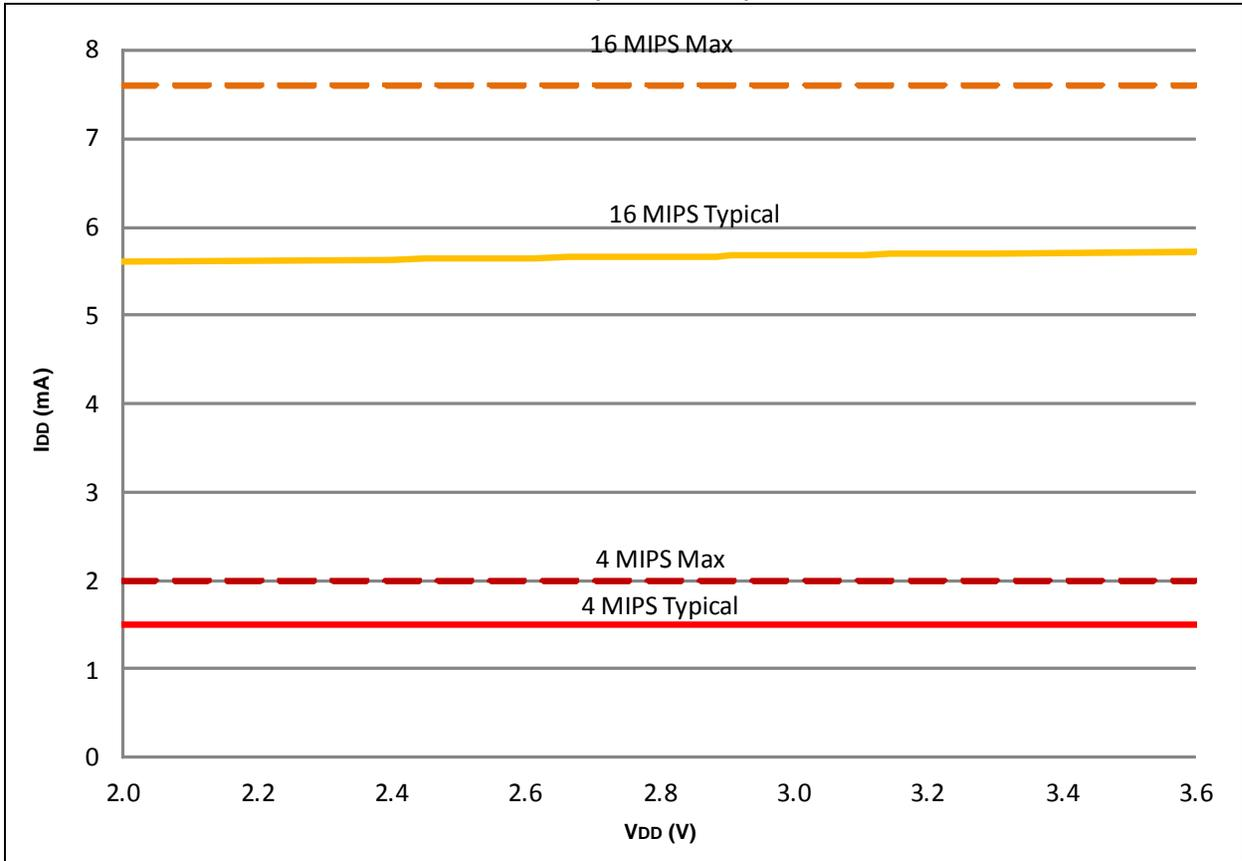
**FIGURE 38-10: I<sub>DD</sub> (RUN MODE) vs. MIPS @ V<sub>DD</sub> = 3.3V**
