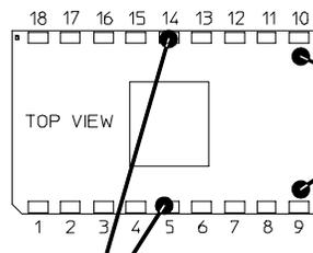
Top of PCB near pin 9 or pin 10 for measurement of maximum product temperature,  $T_{PRODUCT}$
