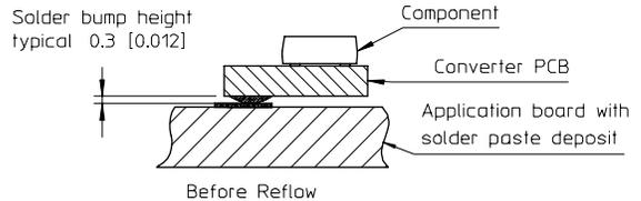
Solder joint thickness:
