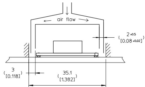
Recommended design of a hot air rework nozzle for manual removal and re-mounting: double wall design directs air flow to solder bump edges only.
