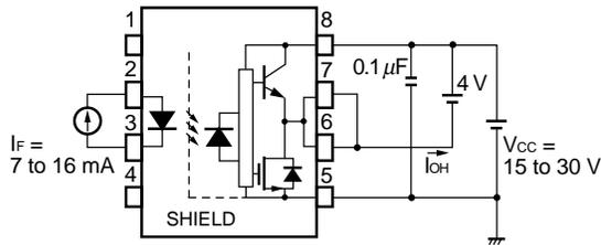
Fig. 2 I<sub>OL</sub> Test Circuit
