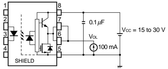
Fig. 5 I<sub>FLH</sub> Test Circuit
