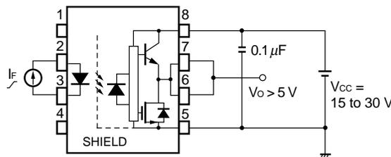
Fig. 6 UVLO Test Circuit
