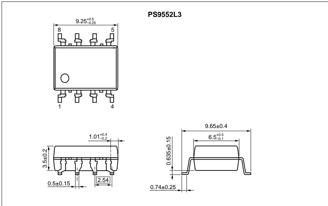
**Lead Bending Type For Long Creepage Distance**
