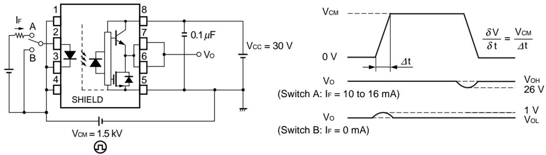
**Remark** CMR Test : Connect pin 1 and pin 4 to the LED common.
