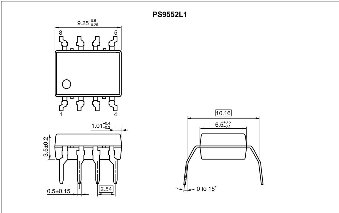
**Lead Bending Type (Gull-wing) For Long Creepage Distance (Surface Mount)**
