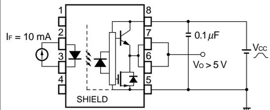
Fig. 7  $t_{PLH}$ ,  $t_{PHL}$ ,  $t_r$ ,  $t_f$  Test Circuit and Wave Forms
