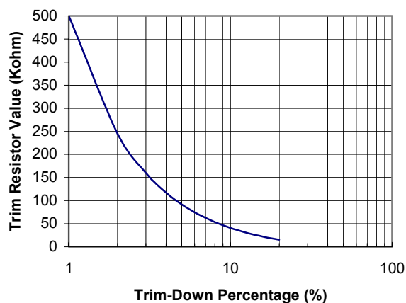
Fig. 18 Trim-Down Resistor Selection
