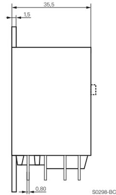
Cover with DIN-snap-on attachment (6.3mm quick connect only)
