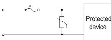
\*In some applications, a polymeric PTC device such as a Tyco Electronics PolySwitch device may be used instead of a fuse to provide a preferred solution.
