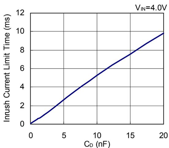
16) Inrush Current Limit Time vs. Input Voltage (E / F Version)
