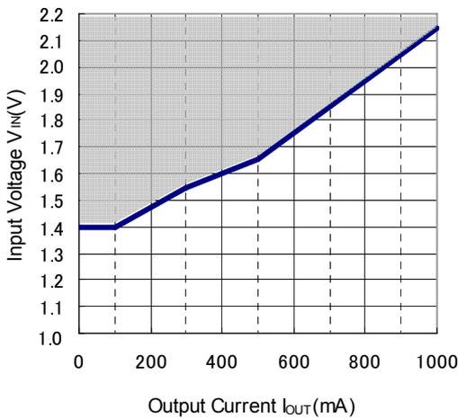
The operation range that can output 0.8V is shown by the hatched area in the graph.
