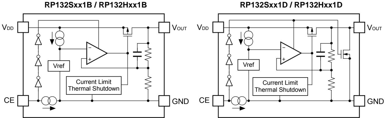
• Fixed Output Voltage Type (TO-252-5-P2 / DFN(PLP)1820-6)
