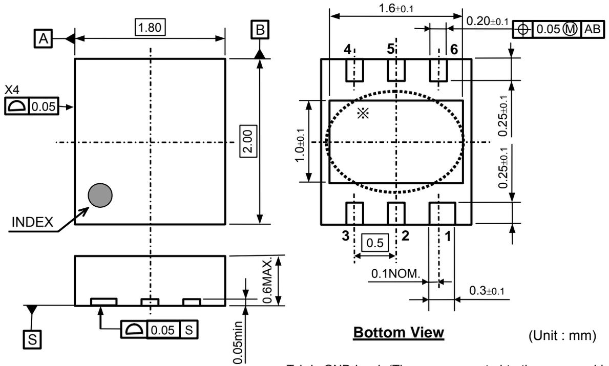
Tab is GND level. (They are connected to the reverse side of this IC.) The tab is better to be connected to the GND, but leaving it open is also acceptable.
