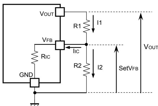
$$I_1 = I_{IC} + I_2 \dots\dots\dots (1)$$
