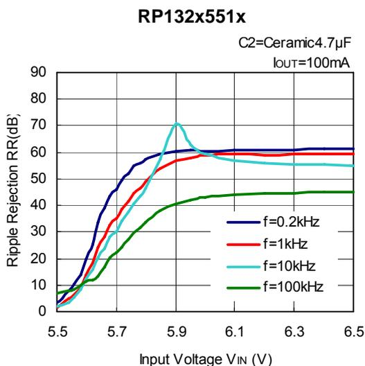
**8) Ripple Rejection vs. Frequency (C1=none, T<sub>opt</sub>=25°C)**
