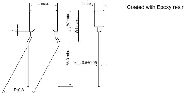
\* Coating extension does not exceed the end of the lead bend.
