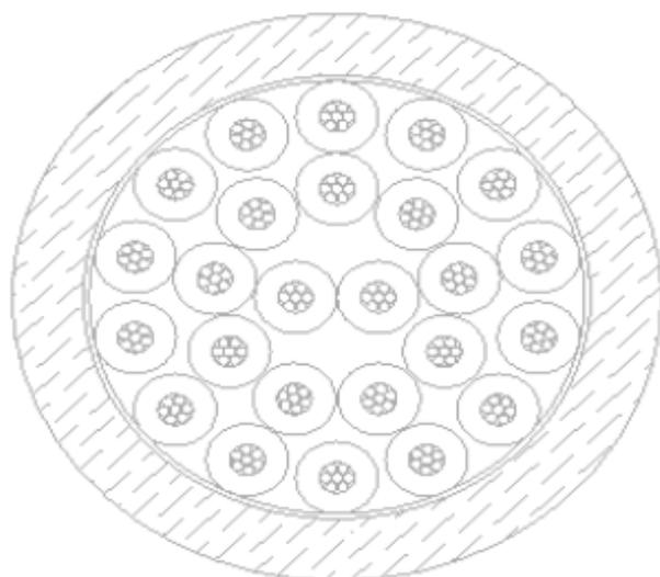
**Description:****Rated Temperature (°C):** -20 ~ 80**Rated Voltage (V):** 250**Flammability Test:** IEC60332-1**Standard:****Manufacture to Def. Stan 61.12 Part 4 & 5****Construction:****Conductor:** Tinned Copper**Conductor Dia. (mm):**  $0.10 \pm 0.008 \times 7$ **Insulation:** PVC**Insulation Dia. (mm):**  $0.7 \pm 0.05 \times 25C$ **Tape:** Mylar Spiral**Coverage:**  $\geq 115\%$ **ID Thread:** Green, White/Green**A rip cord :** 210 D**Jacket:** FR-PVC**Outer Dia. (mm):**  $5.5 \pm 0.1$
