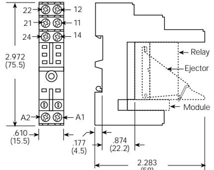
Ejector/Hold-Down Spring RT16016<sup>3</sup>
