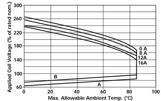
A: Coil temperature = Ambient temperature.
