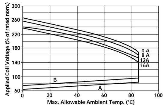
A: Coil temperature = Ambient temperature.
