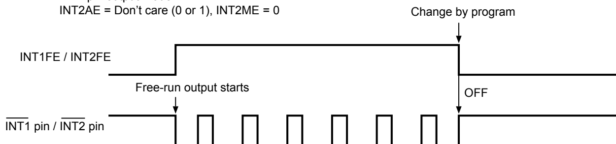
Figure 27 Output Timing of User-set Frequency
