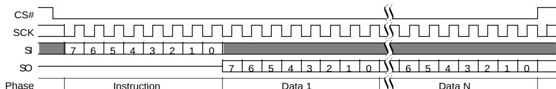
Figure 10.70 Password Read (PASSRD E7h) Command Sequence
