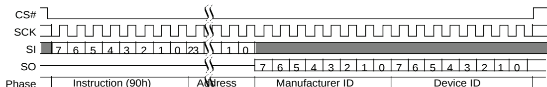
Figure 10.1 READ_ID (90h) Command Sequence
