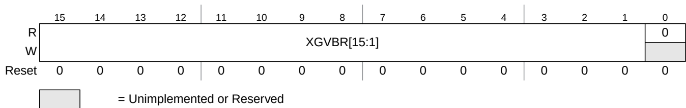
Figure 5-5. XGATE Vector Base Address Register (XGVBR)
