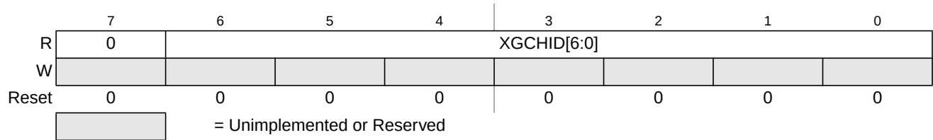
Figure 5-4. XGATE Channel ID Register (XGCHID)
