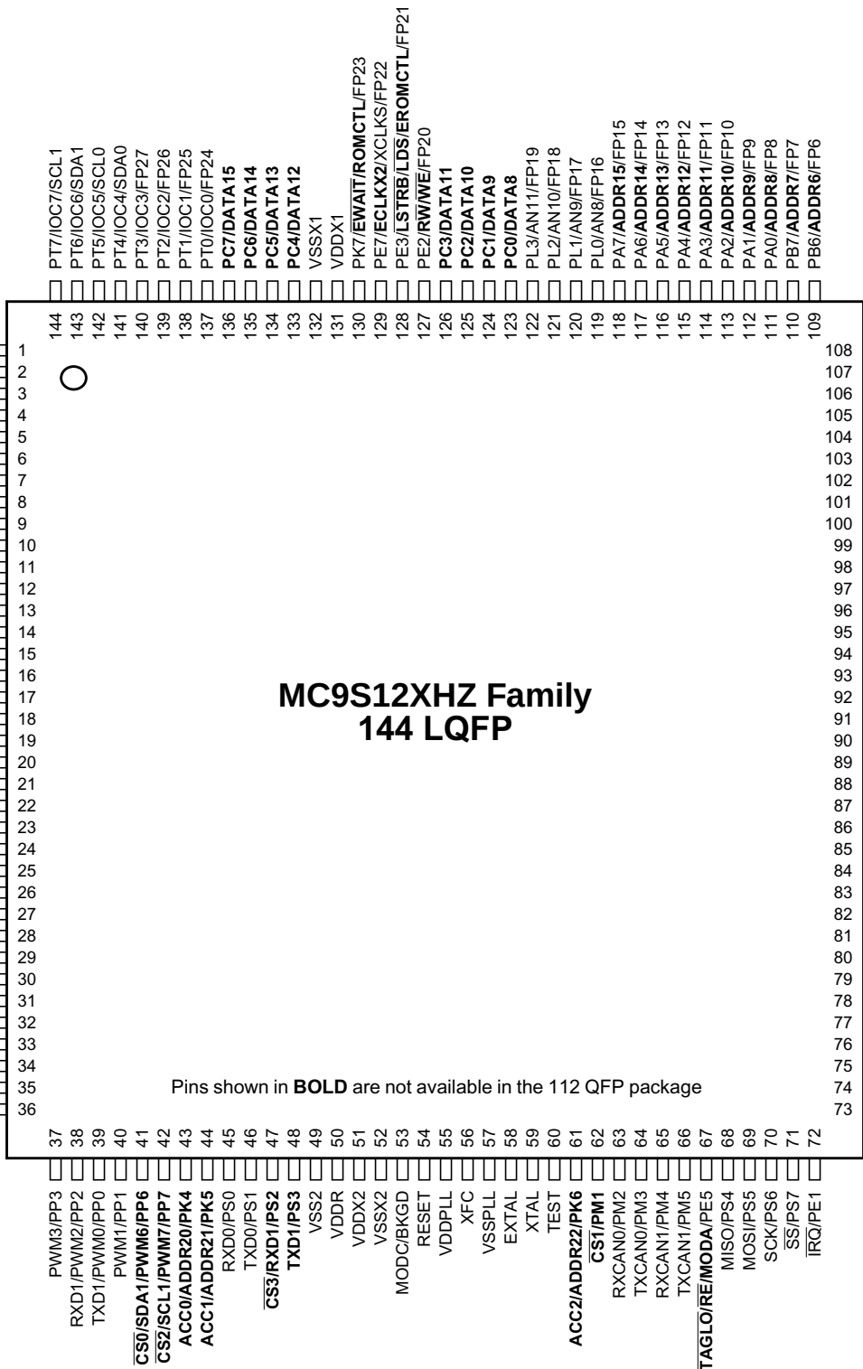
Figure 1-4. MC9S12XHZ Family 144 LQFP Pin Assignment
