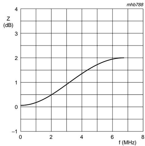
Fig 27. C<sub>B</sub>-C<sub>R</sub> low-pass filter frequency response
