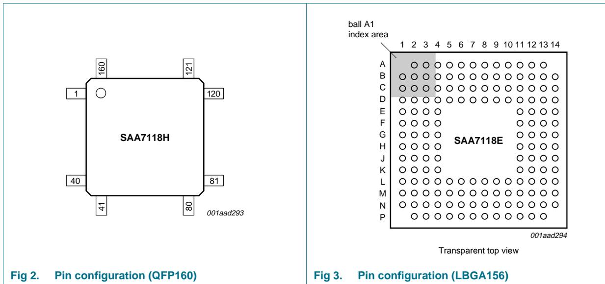
Fig 2. Pin configuration (QFP160)
