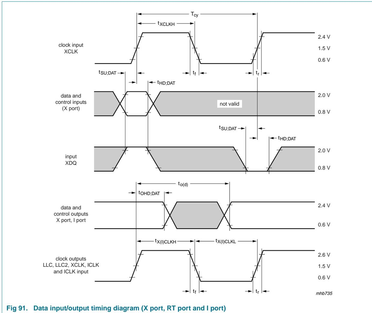
Fig 91. Data input/output timing diagram (X port, RT port and I port)
