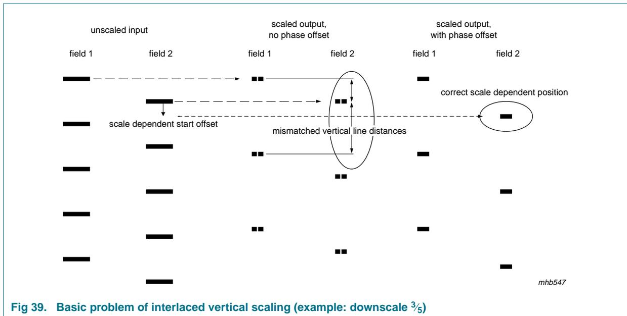
Fig 39. Basic problem of interlaced vertical scaling (example: downscale 3/5)
