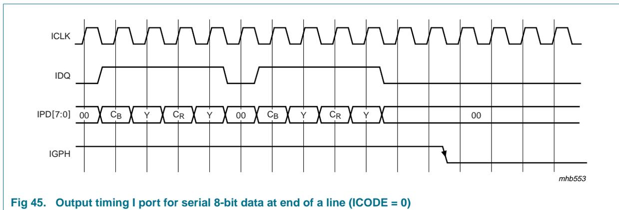
Fig 45. Output timing I port for serial 8-bit data at end of a line (ICODE = 0)
