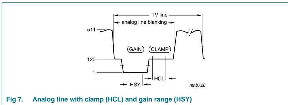
Fig 7. Analog line with clamp (HCL) and gain range (HSY)
