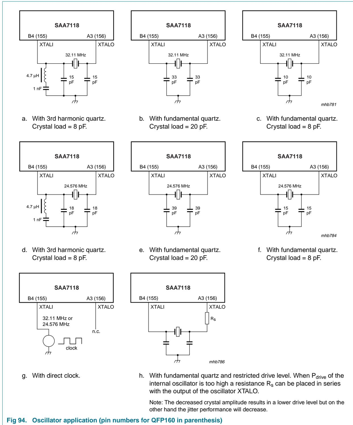
Fig 94. Oscillator application (pin numbers for QFP160 in parenthesis)
