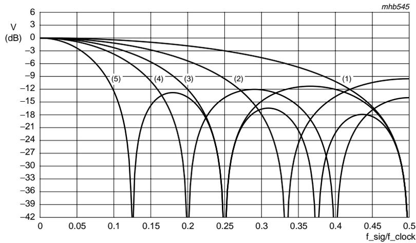
$XC2\_1 = 0$ ; Zero's at  $f = n \times \frac{I}{XACL+1}$  with  $XACL = (1), (2), (3), (4)$  or  $(5)$
