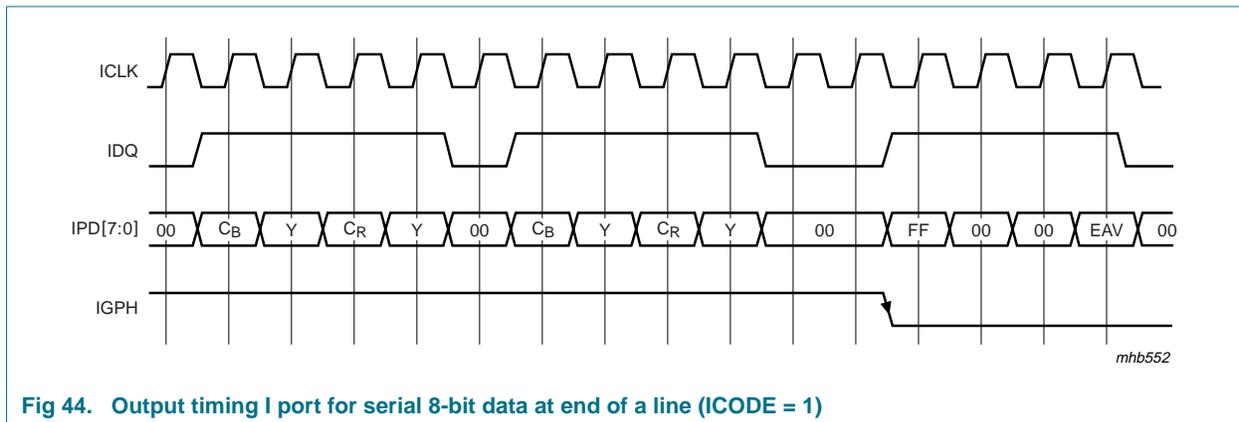
Fig 44. Output timing I port for serial 8-bit data at end of a line (ICODE = 1)
