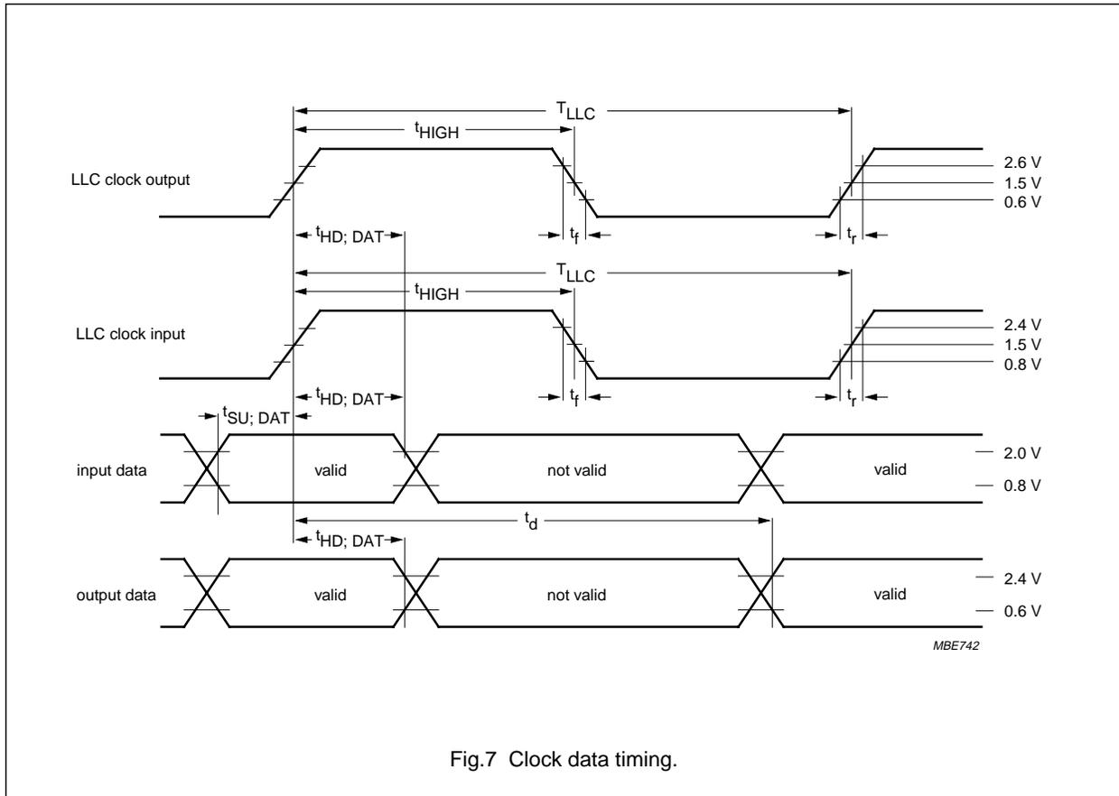
Fig.7 Clock data timing.
