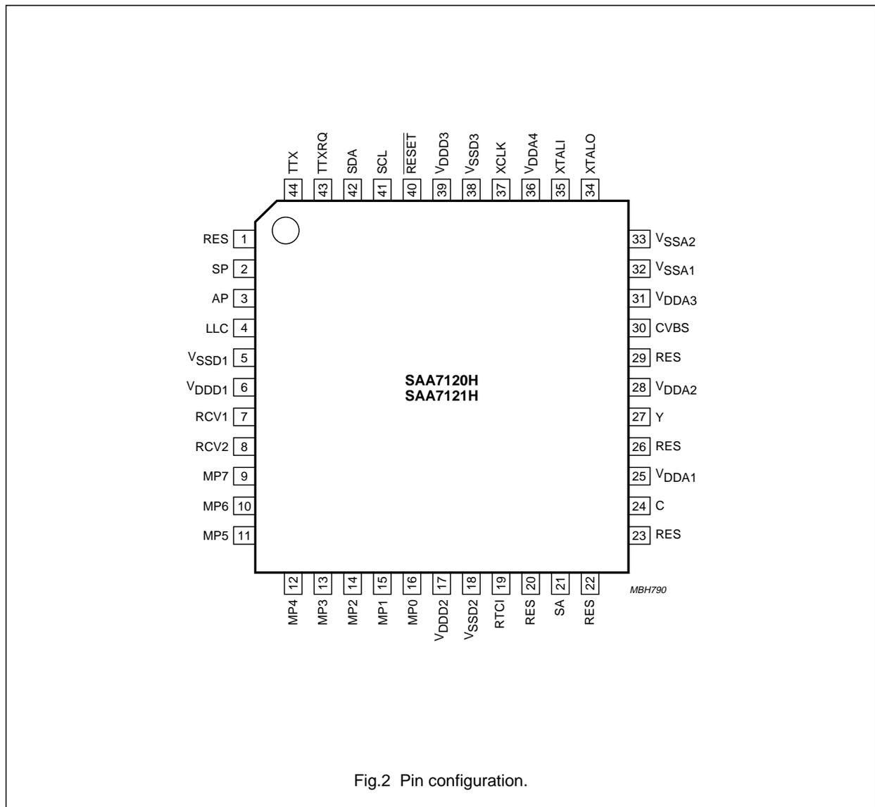
Fig.2 Pin configuration.
