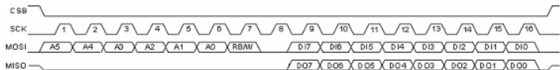
Figure 9. SPI frame format for two 8 bit words.
