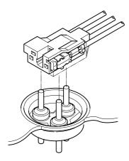
This three circuit connector is used to connect cluster pins (2.3mm in diameter) to the leads of a motor hermetically sealed in a compressor of a refrigerator or a freezer. The contacts and housing are especially designed and made of high-quality materials for high heat resistance and superior durability.
