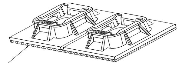
ADHESIVE BACKING: RUBBER BASED ADHESIVE PRESSURE SENSITIVE FOAM TAPE 0.04 [1.0] THICK WITH A PROTECTIVE LINER. MOUNT IS DESIGNED TO SUPPORT 0.50 lbs (227g) MAX. WEIGHT ON A CLEAN DRY SMOOTH SURFACE.
