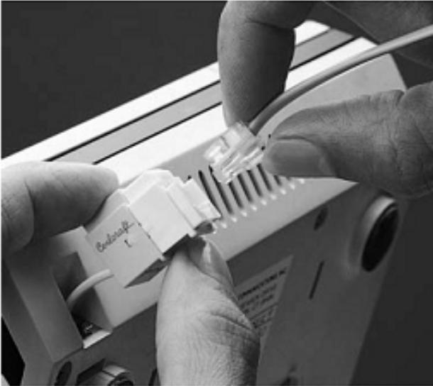
Eliminating common mode EMI from telephone lines, handset cords, and LANs can be done quickly and easily with these plug-in filter modules.
