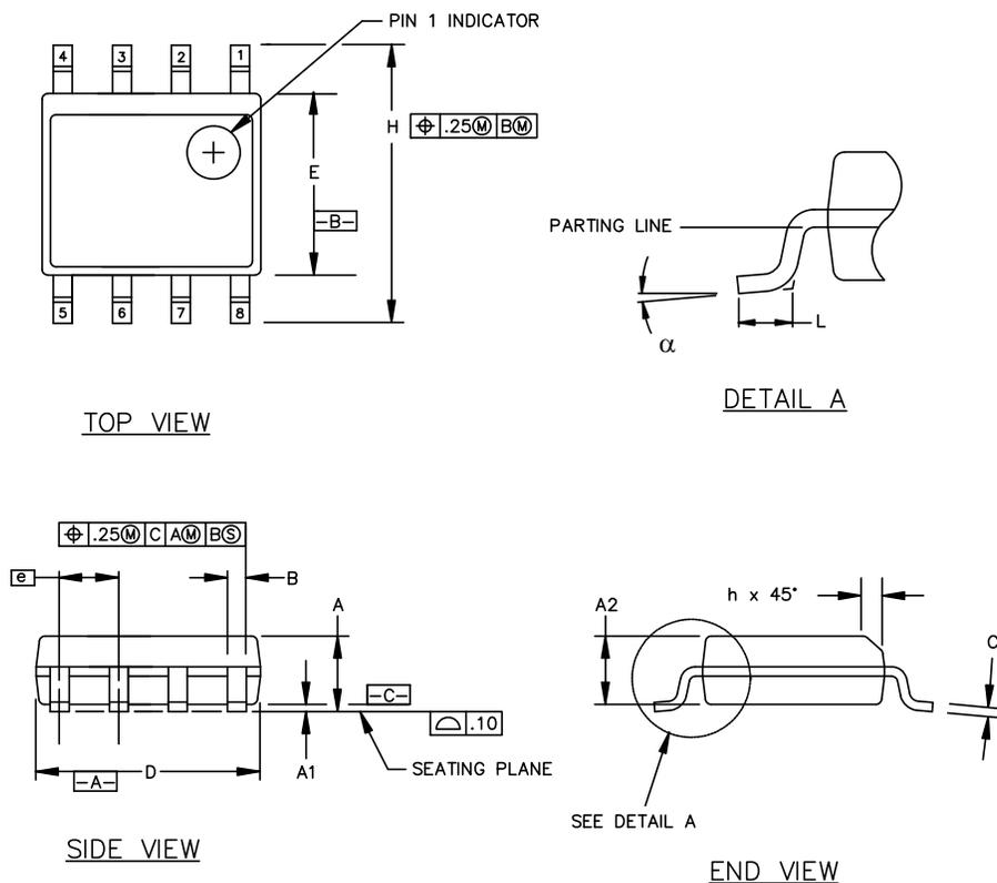
**Figure 14. 8-pin Small Outline Integrated Circuit (SOIC) Package**
