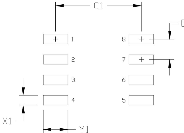
Figure 15. PCB Land Pattern: 8-Pin Narrow Body SOIC
