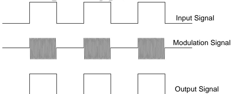
**Figure 4. Modulation Scheme**
