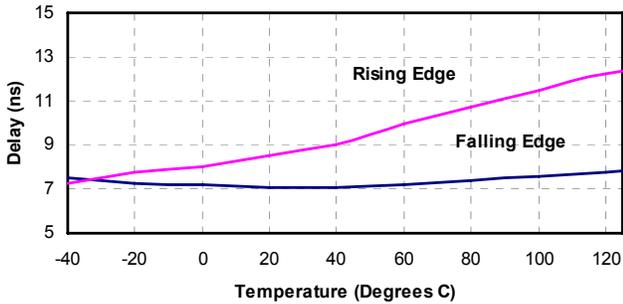
**Figure 11. Propagation Delay vs. Temperature 2.5 V Operation**
