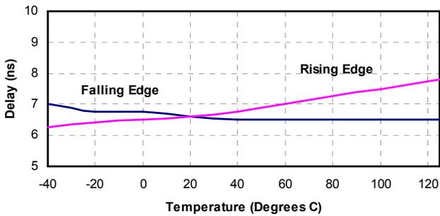
**Figure 10. Propagation Delay vs. Temperature 3.3 V Operation**
