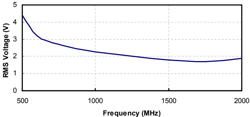
Figure 16. RMS Common Mode Voltage vs. Frequency
