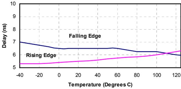
**Figure 9. Propagation Delay vs. Temperature 5 V Operation**
