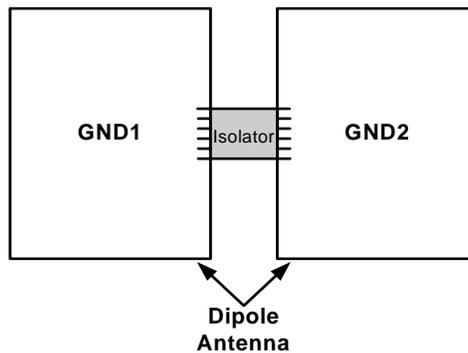
**Figure 15. Dipole Antenna**
