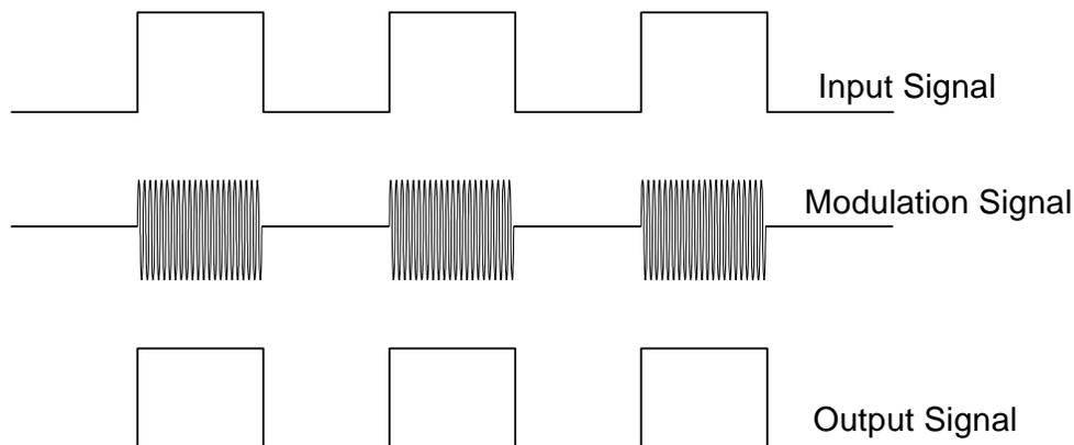
**Figure 12. Modulation Scheme**
