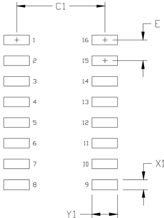
**Figure 20. 16-Pin Narrow Body SOIC PCB Landing Pattern**
