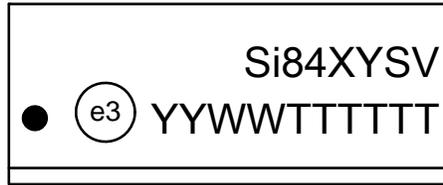
Figure 22. 16-Pin Narrow Body SOIC Top Marking
