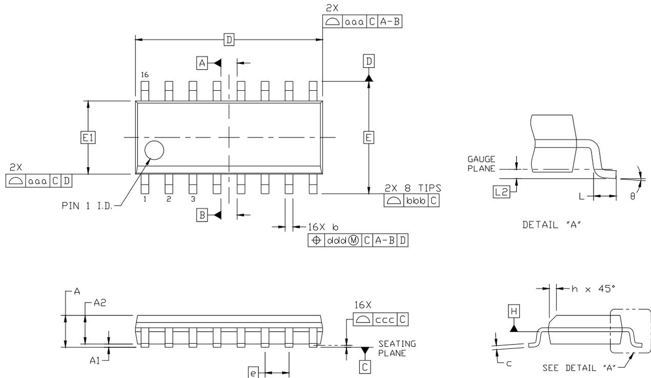
**Figure 19. 16-pin Small Outline Integrated Circuit (SOIC) Package**
