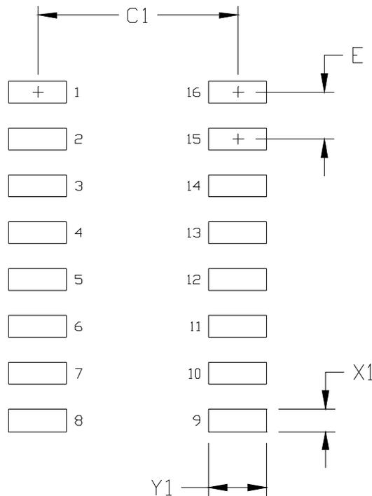
**Figure 17. 16-Pin Narrow Body SOIC PCB Land Pattern**
