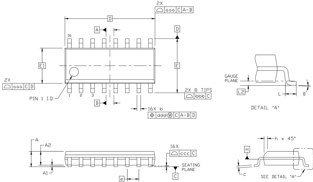
Figure 16. 16-pin Small Outline Integrated Circuit (SOIC) Package
