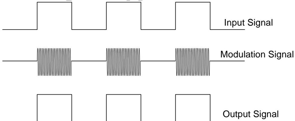
**Figure 4. Modulation Scheme**
