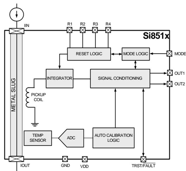
Figure 3. Si851x (Ping Pong Output) Block Diagram
