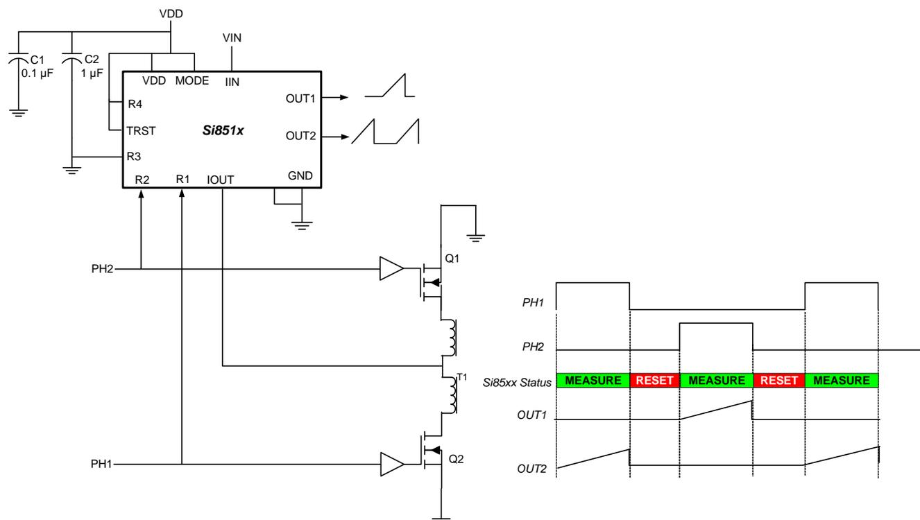
Figure 19. Push-Pull Example Using Default  $t_R$  Value
