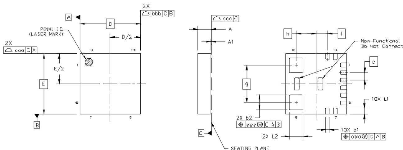
Figure 22. 12-Pin QFN Package Diagram
