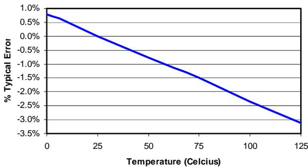
**Figure 6. Differential Temperature Calibration Error**
