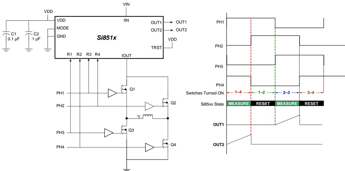
**Figure 18. Full-Bridge Converter**
