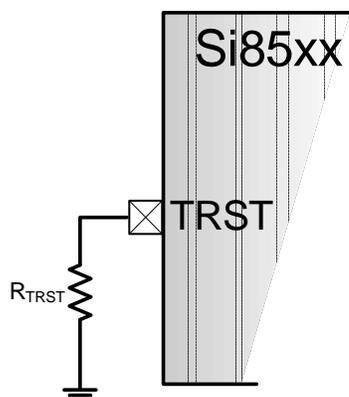
Figure 5. Programming Reset Time ( $t_R$ )
