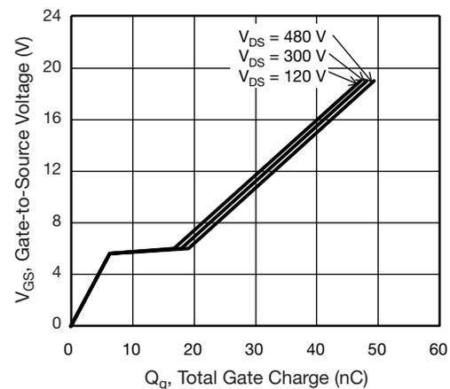
**Fig. 6 - Typical Gate Charge vs. Gate-to-Source Voltage**
