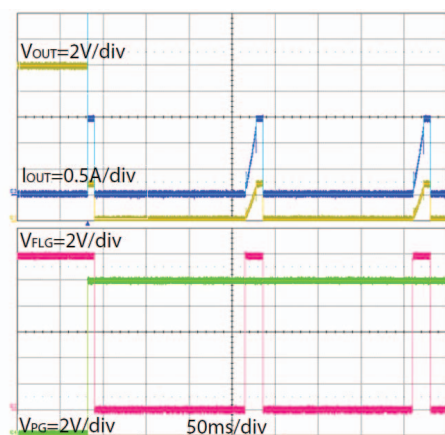
Fig. 31 - SiP32429 Re-Starts after ~ 150 ms during Fault Condition
