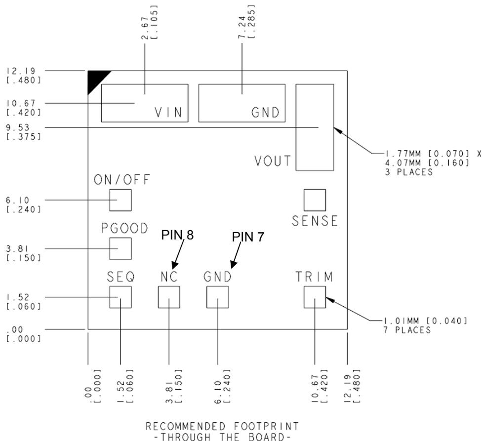
Dimensions are in millimeters and (inches).
