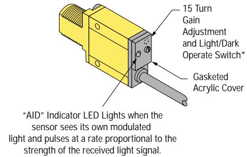
"AID" Indicator LED Lights when the sensor sees its own modulated light and pulses at a rate proportional to the strength of the received light signal.
